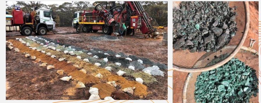
Drill rig at HWRC003 (left) with sieved chips showing contrast between mineralised structure and fuchsite alteration halo (right)
