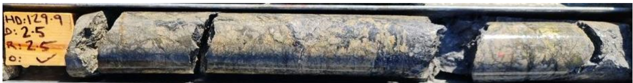
Figure 1 Core section from third hole – sulphides (pyrite/chalcopyrite) in yellow in intensely veined and brecciated stockwork in sandstone.
