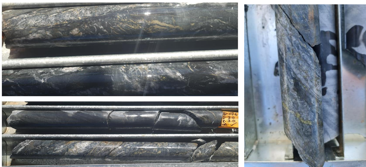
Figure 4 – RDD001 (a) Typical core with sulphides around 117.6m; (b) Chalcopyrite mineralisation at 430m.
