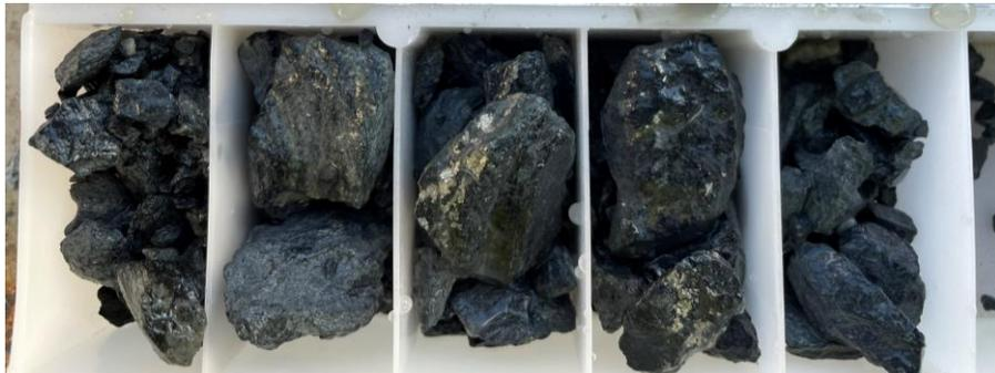
RC drill chips with altered and sulphidic basalts – WJRC0038
