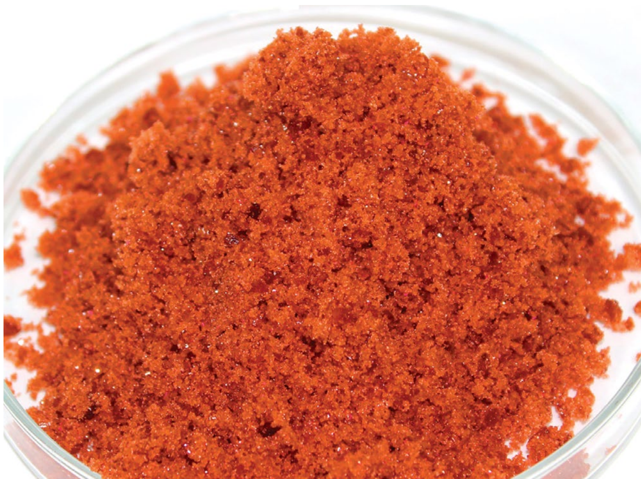
Figure 3 – Cobalt sulphate heptahydrate crystals
