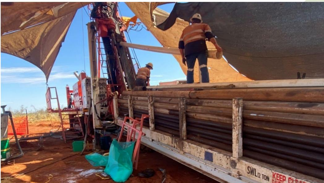
Figure 1: Drilling contractor Eagle Drilling NQ installing surface casing in KNRDD002 at “Twin Peaks” West.
