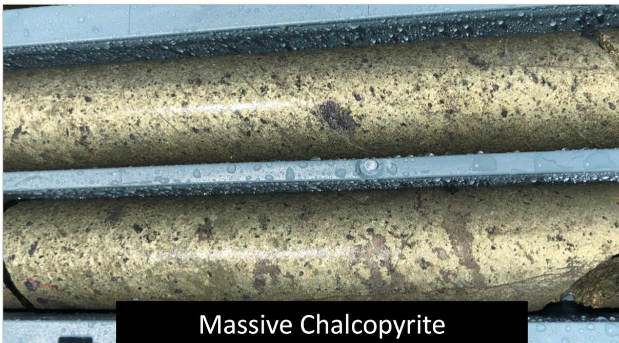
Figure 3: Close-up of massive chalcopyrite-pyrite zone in hole KJCD481D3
