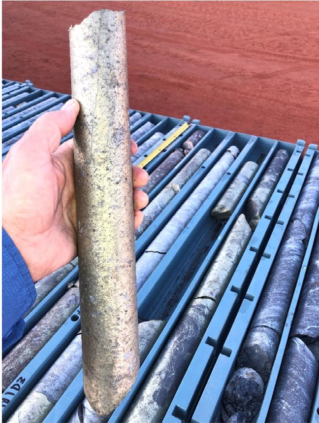
Figure 1: Massive copper-sulphide Intersection in in hole KJCD481D3
