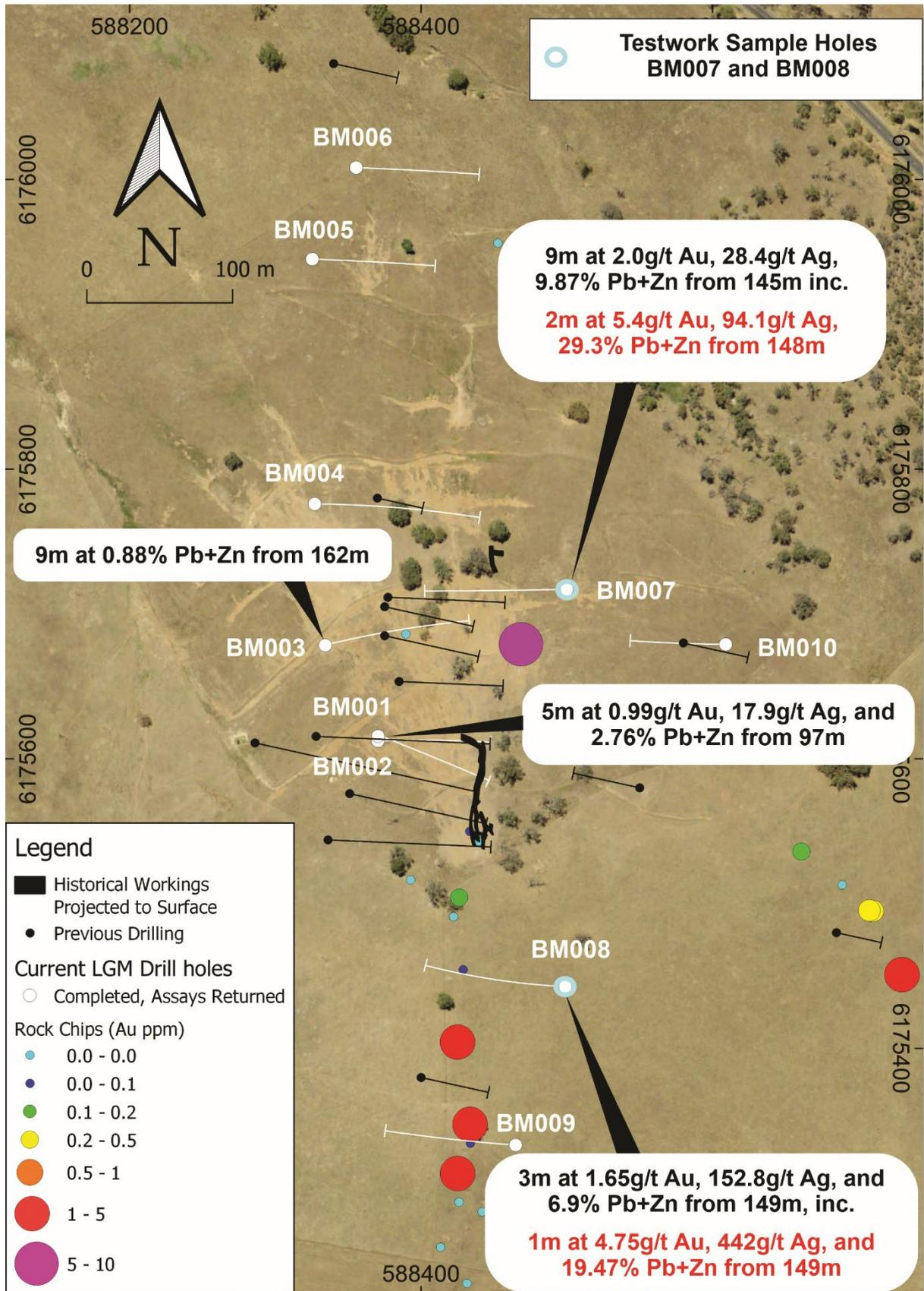
Figure 2: Mt Felstead Prospect test-work drill hole locations.
