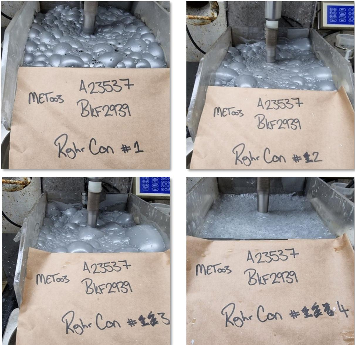
**Figure 1:** Mt Felstead Prospect rougher flotation concentration stages one to four (BKF2939)
