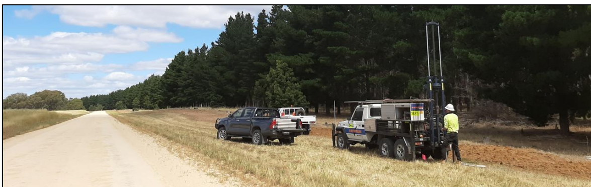
Figure 3 – Push Tube/core drilling in progress
