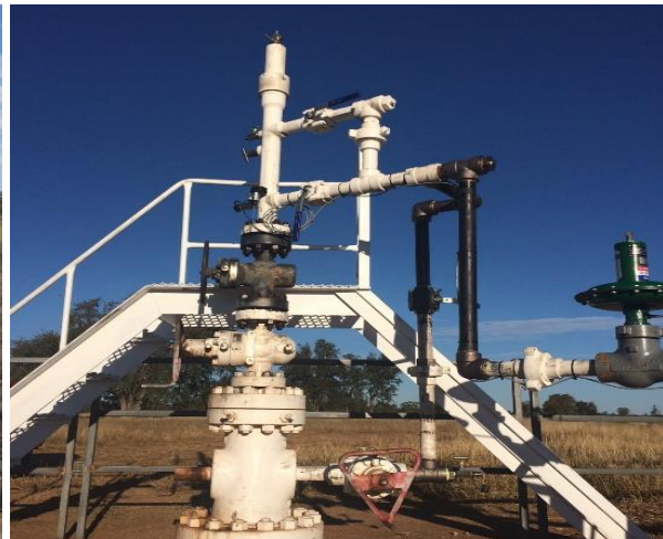
Fig 4: Plunger Lift Installation (June 2021)
