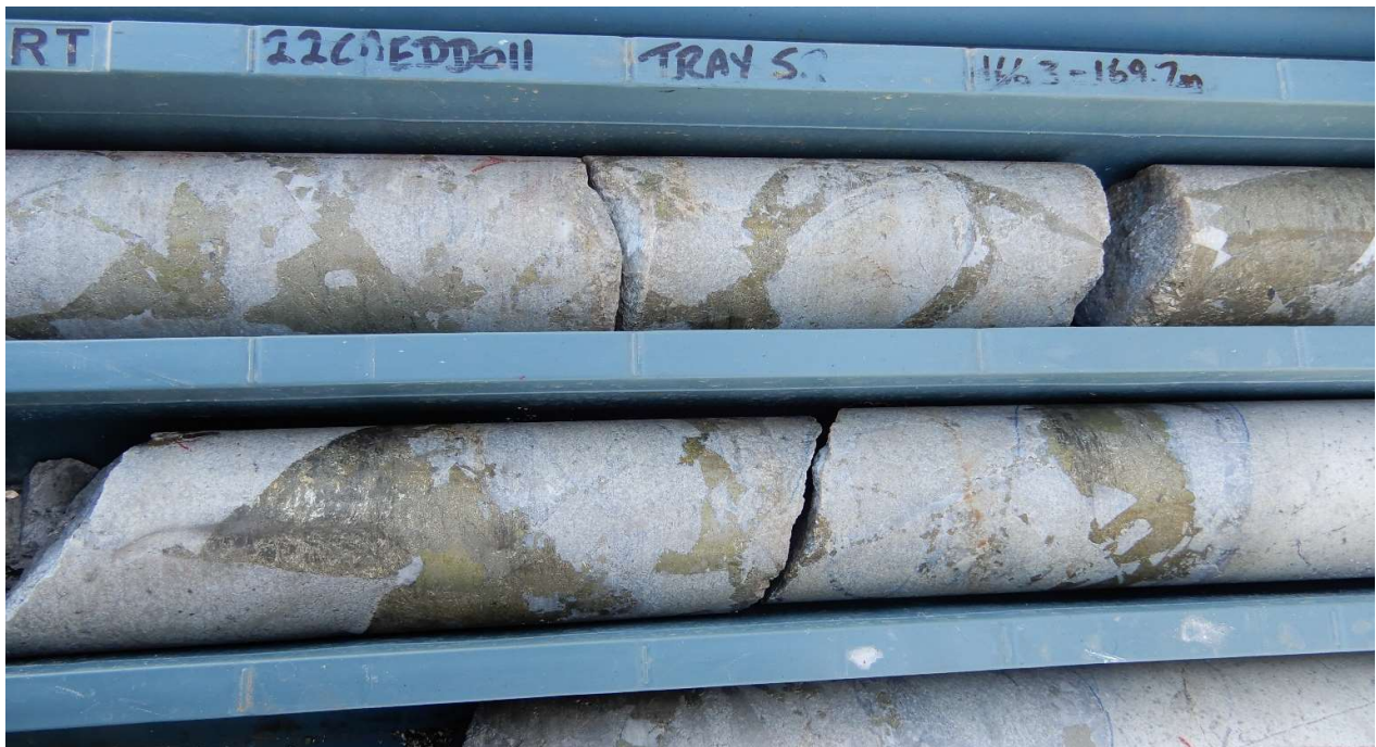
Fig 9 HQ Core photo hole 22CAEDD0011, 167m Chalcopyrite -pyrite , minor quartz calcite infill between blocks diorite in clast supported infill breccia. Primary zone 166m-168m assays 2m @ 1.63% Cu, 1.24 g/t Au, 28.5 g/t Ag, 15.48 % S.
