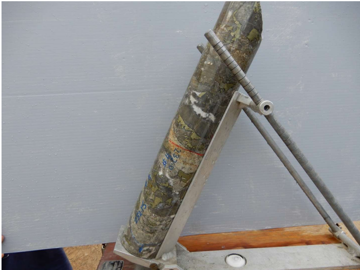
Fig 15 HQ Core photo hole 22CAEDD0011, 232m. HQ Core Photo in core frame oriented relative to actual drillhole surveyed position, looking north.Tabular, slab-like clasts dipping to south east with infill chalcopryite-pyrite-quartz-calcite. Primary zone 231m-233m assays 2m @ 4.01% Cu,0.48 g/t Au, 48.4 g/t Ag, 5.99 % S.
