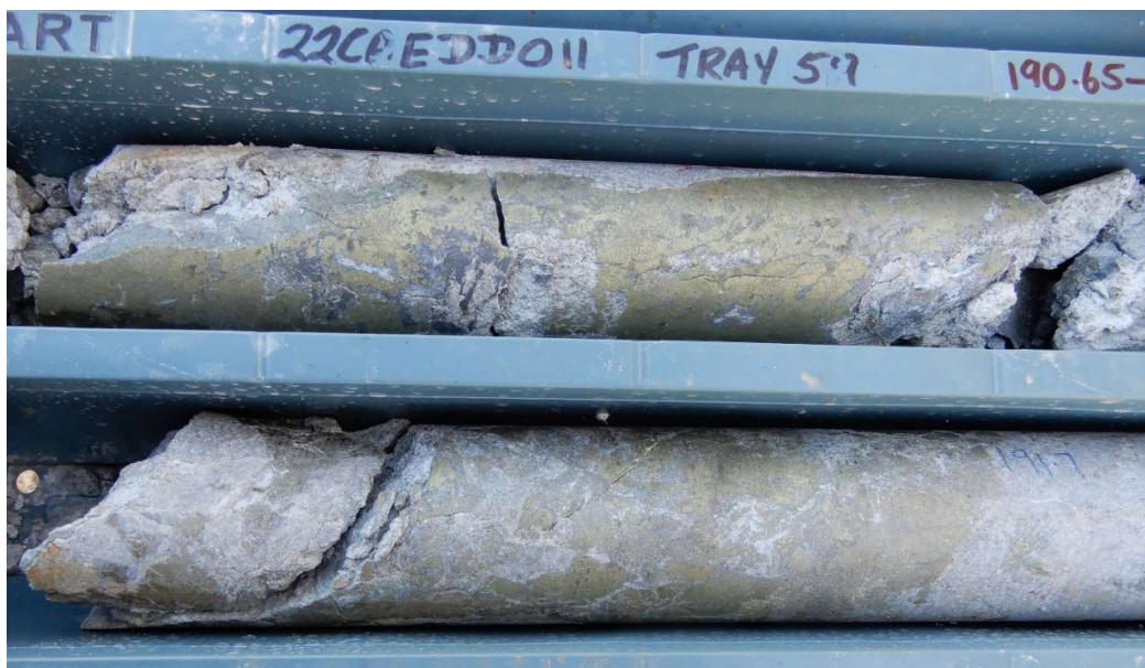
Fig 12 HQ Core photo hole 22CAEDD0011, 191m Chalcopyrite -pyrite , quartz calcite semi massive sulphide vein cutting diorite. Primary zone 190m-192m assays 2m @ 5.45% Cu, 5.95 g/t Au, 132.1 g/t Ag, 16.14 % S.
