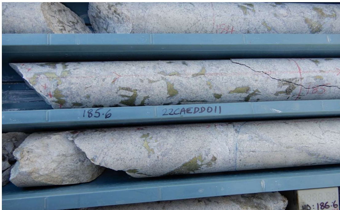
Fig 11 HQ Core photo hole 22CAEDD0011, 185m Chalcopyrite -pyrite , quartz calcite infill between blocks diorite in clast supported breccia. Primary zone 185m-187m assays 2m @ 1.66% Cu, 0.26 g/t Au, 24.55g/t Ag, 7.03 % S.
