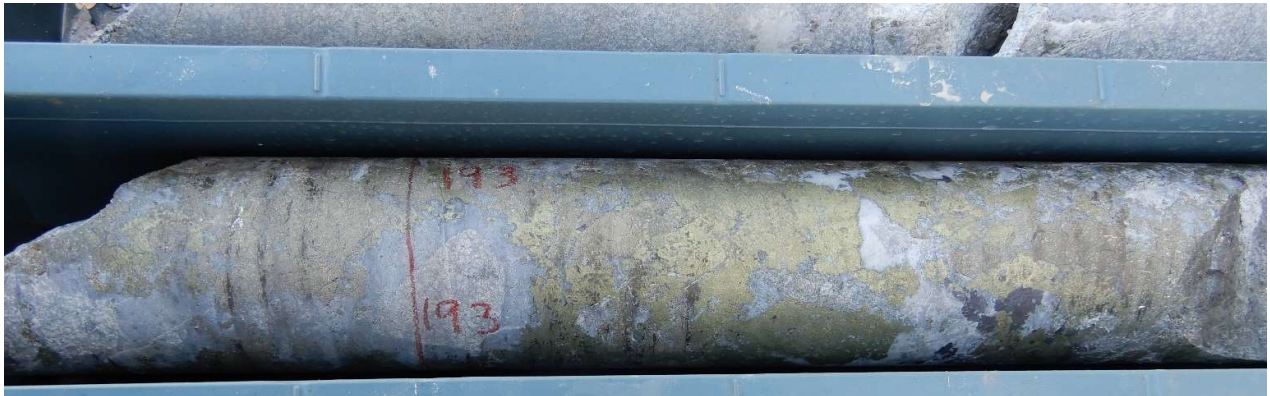
Fig 14 HQ Core photo hole 22CAEDD0011, 193m , massive chalcopryite -pyrite , quartz calcite feeder like vein cutting diorite. Primary zone 192m-193m assays 1m @ 1.57% Cu,1.75 g/t Au, 43.6 g/t Ag, 8.68 % S.
