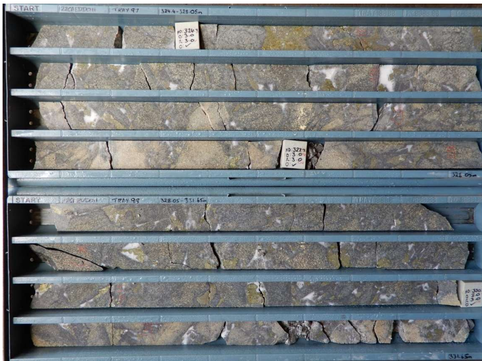
Fig 17 HQ Core photo hole 22CAEDD0011, 324.4 -331.65m Chalcopyrite -pyrite , quartz calcite infill in diorite breccia. Primary zone 324m-332 assays 8m @ 1,71% Cu, 0.33 g/t Au, 25.7 g/t Ag, 7.76 % S.
