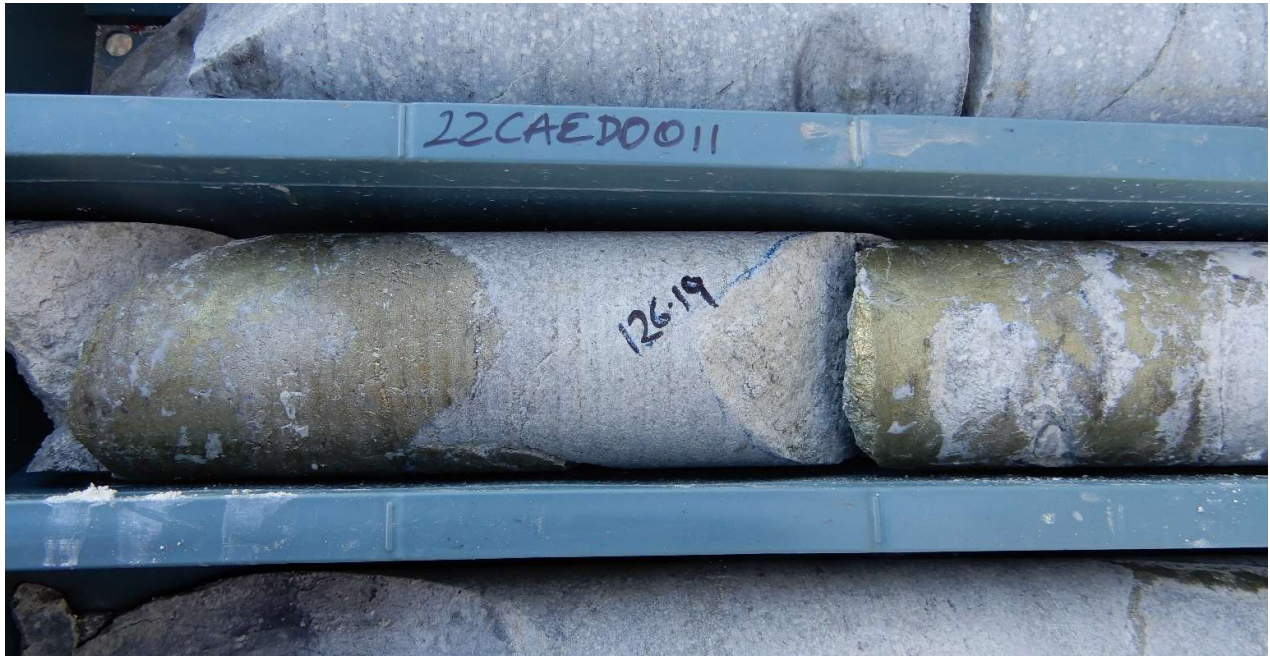
Fig 8 HQ Core photo hole 22CAEDD0011, 126m Chalcopyrite -pyrite veins and aggregations in diorite . Primary zone 126m-127m assays 1m @ 2.50% Cu, 3.73 g/t Au, 66.9 g/t Ag, 10.82 % S.
