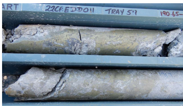
Chalcopyrite rich, possible sulphide feeder structure at 191m, CAE Hole # 11 grading 5.45% Cu, 5.95 g/t Au, 132.1 g/t Ag.
