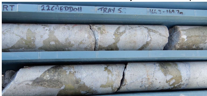
Sukphidic breccia at 166m – 168m grading 1.63% Cu, 1.24 g/t Au, 28.5 g/t Ag.
