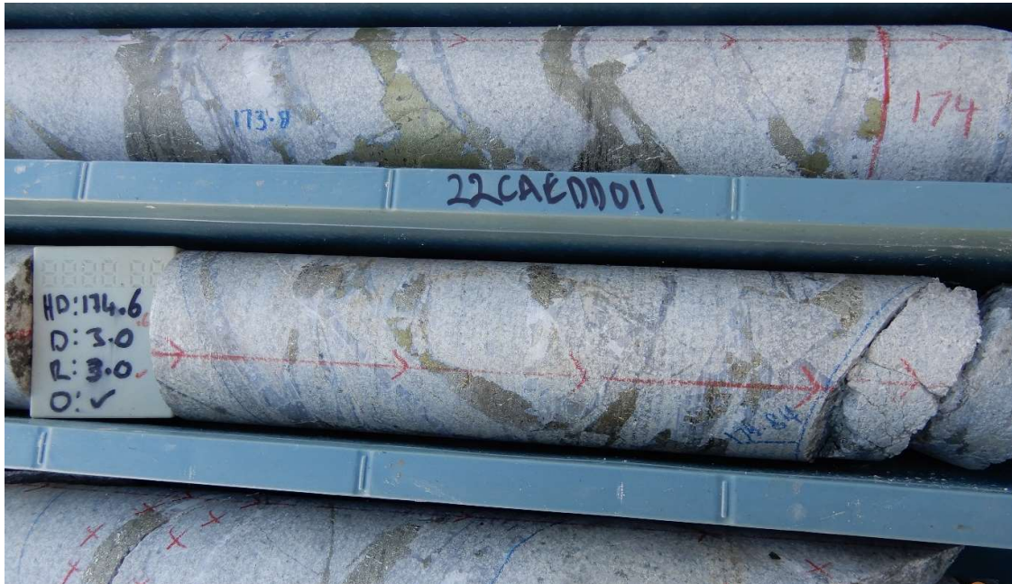
Fig 10 HQ Core photo hole 22CAEDD0011, 174m Chalcopyrite -pyrite , quartz calcite infill between blocks diorite in clast supported breccia. Primary zone 173m-176m assays 3m @ 1.17% Cu, 0.21 g/t Au, 22.73 g/t Ag, 8.31 % S.
