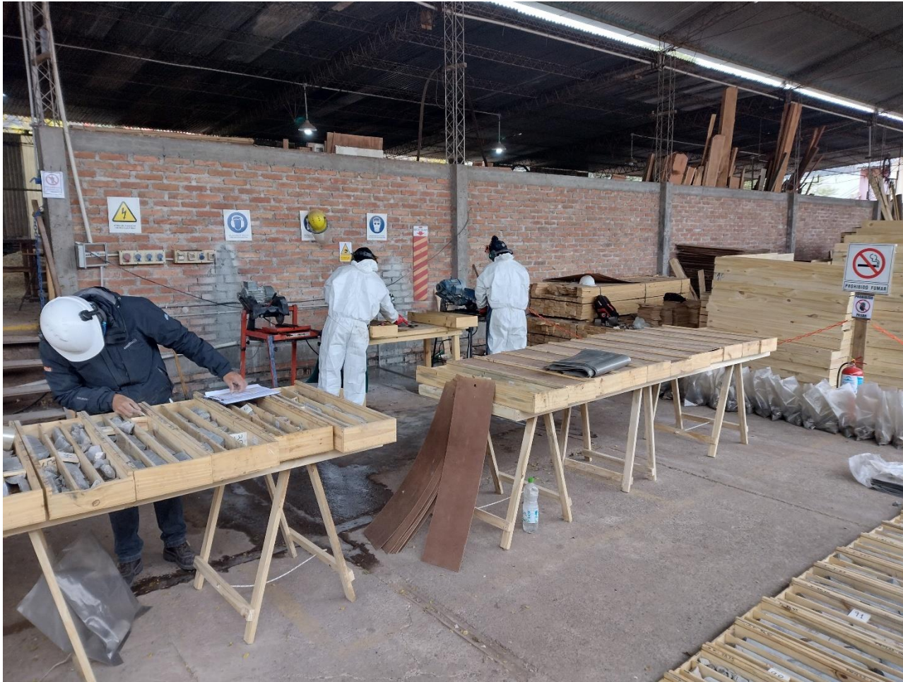
Drill core from Santa Ines Project being cut and logged
