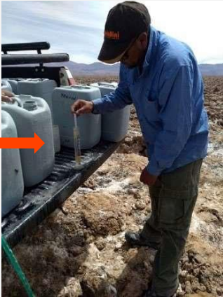
Relative density of brine measured
