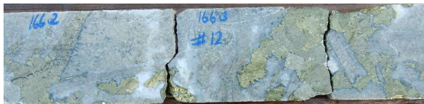
Chalcopyrite – pyrite-quartz – calcite infill between angular clasts of sericite altered diorite. CAE hole # 12, 166.3m. Interval 166m-167m grading 3.05% Cu, 0.56 g/t Au, 55.2 g/t Ag, 9.62% S,
