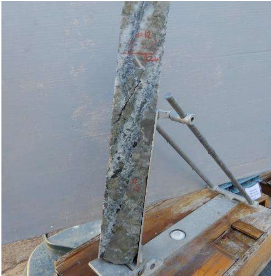
Fig 16. HQ half Core oriented in Core Orienting Frame, hole drilling north at 80 degrees, looking south-east. Sheeted veins of quartz-calcite-pyrite-black sphalerite and chalcopyrite-minor galena. Veins cut a breccia dominated by hornfels clasts. Vein has east west strike (100-280 magnetic bearing dipping 70 degrees to north). Hole 22CAEDD0012, 224m, Interval 223m-225m 2m grading 1.53% Cu, 2.73g/t Au, 86.9 g/t Ag, 4.95% S, 2315 ppm As, 635 ppm Pb, 1159 ppm Sb, 5272 ppm Zn.
