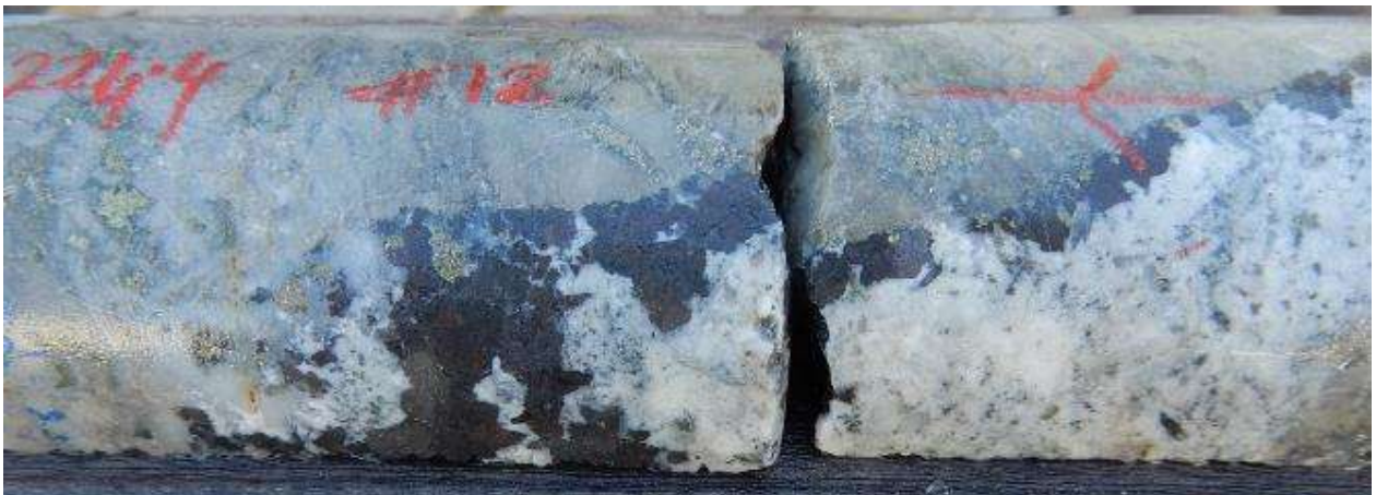
Fig 15. Close up HQ half core black sphalerite rich vein cutting a breccia dominated by hornfels clasts. Quartz-calcite-sphalerite-pyrite-chalcopyrite bearing vein. CAEDD0012, 224m.4, Interval 224m-225m 1m grading 0.91% Cu, 2.37g/t Au, 76 g/t Ag, 4.51% S, 2712 ppm As, 615 ppm Pb, 2712 ppm Sb, 8202 ppm Zn.
