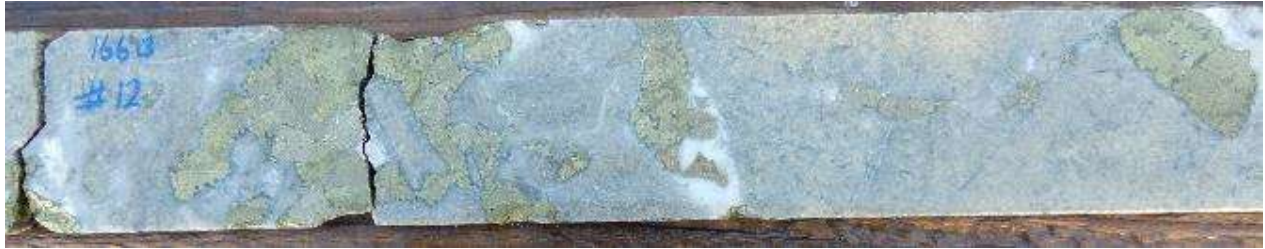
Fig 11. HQ Core photos hole 22CAEDD0012, 166.0m, Chalcopryite – pyrite-quartz – calcite infill between angular clasts of sericite altered diorite. Interval 166m-167m grading 3.05% Cu, 0.56 g/t Au, 55.2 g/t Ag, 9.62% S
