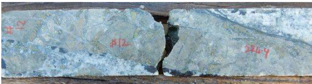
Fig 17. Close up HQ half sheeted veins cutting a breccia dominated by hornfels clasts. Two sheeted veins with intervening sericite altered hornfels dominated breccia. CAEDD0012, 224m.4 , Interval 224m-225m 1m grading 0.91% Cu, 2.37g/t Au, 76 g/t Ag, 4.51% S, 2712 ppm As, 615 ppm Pb, 2712 ppm Sb, 8202 ppm Zn.
