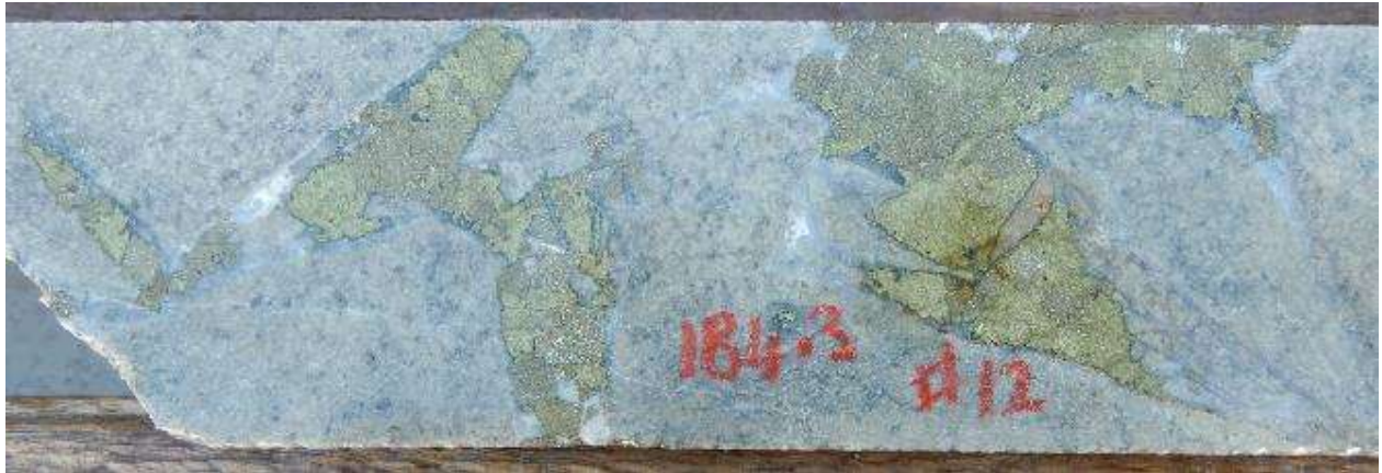
Fig 13 HQ Half Core photos hole 22CAEDD0012, 184.3, Chalcopyrite pyrite-calcite infill in monomict crackle brecciated diorite.. Interval 184m-185m assays 1m @ 2.36% Cu, 0.22 g/t Au, 33.5 g/t Ag, 6.38 % S
