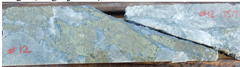
Contact between chalcopyrite- pyrite-quartz calcite vein infill and sericite-calcite altered diorite breccia. CAE hole # 12, 175.7m. Interval 175m-176m grading 2.45% Cu, 0.54 g/t Au, 50.6 g/t Ag, 7.86% S,
