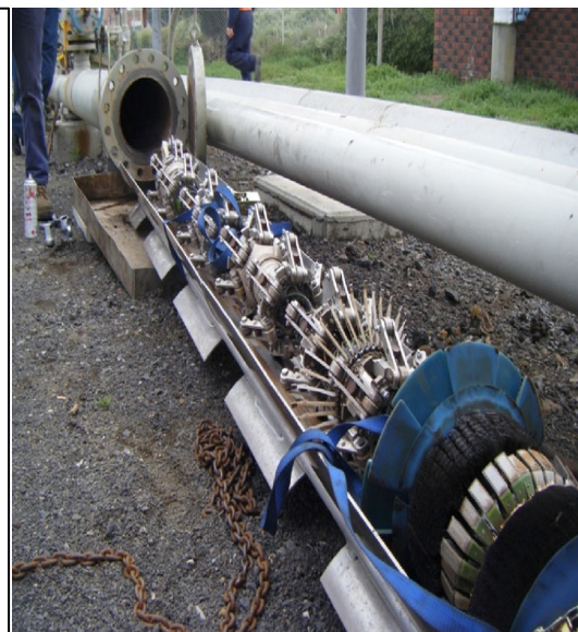
Figure 5 - Intelligent Pig
