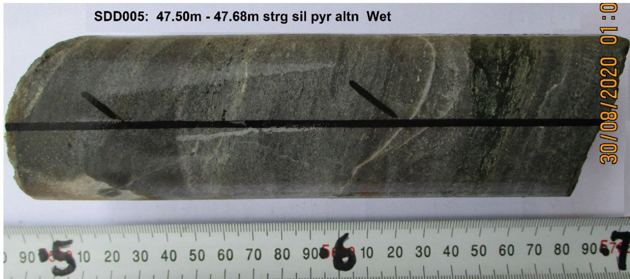
Figure 11. 2020 diamond core from the Steam Engine Lode (DDD005, 47-48m, assayed 4.1 g/t Au).
