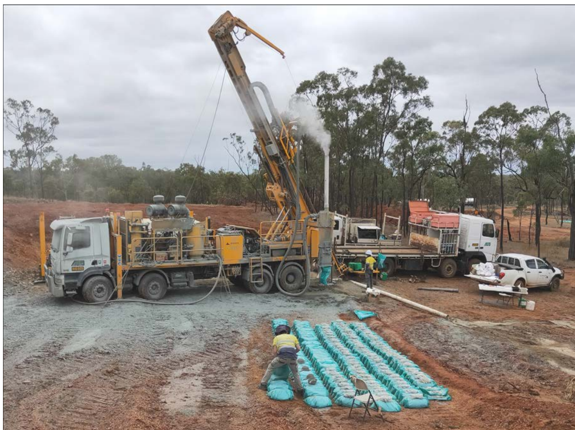
Figure 10. Reverse Circulation drilling and sampling at the Steam Engine Lode
