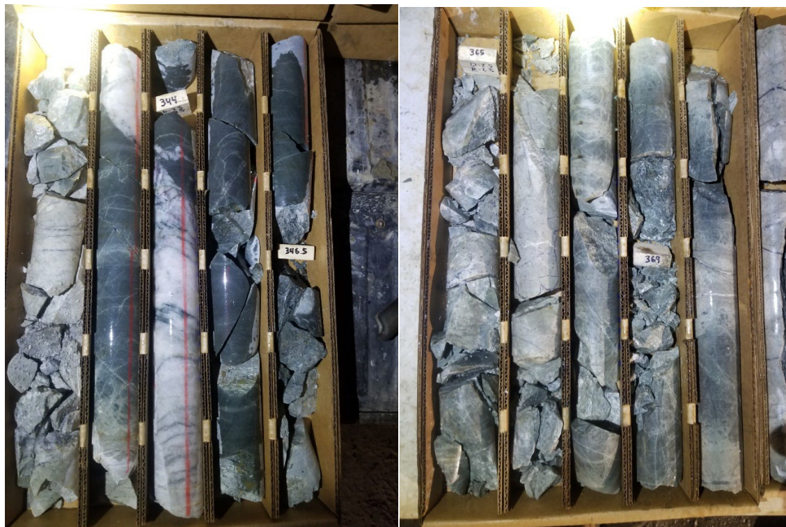
Figure 4 Section of core showing the large 3.7 metre mineralized vein material. Vein is intensely quartz sericite altered with stringers of sphalerite, galena, and pyrite sulfidation, which is where the gold is associated.
