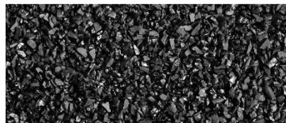
In collaboration with US partner, about to start trials of new high capacity P adsorption pellet to treat stormwater and agricultural run off
