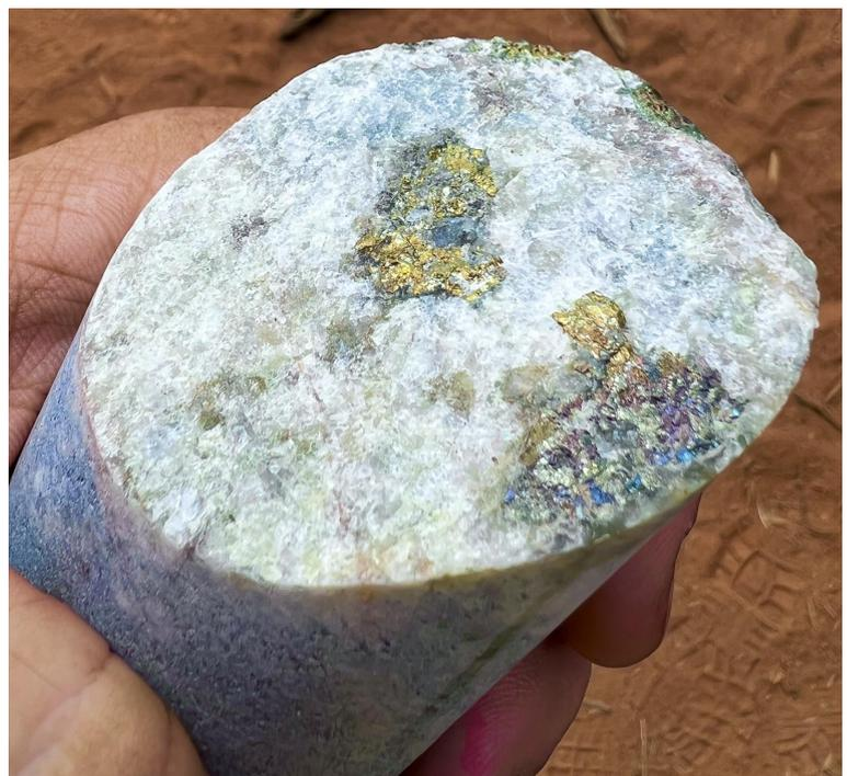
**Figure 1:** Bornite mineralisation in drill core (240m Depth)
