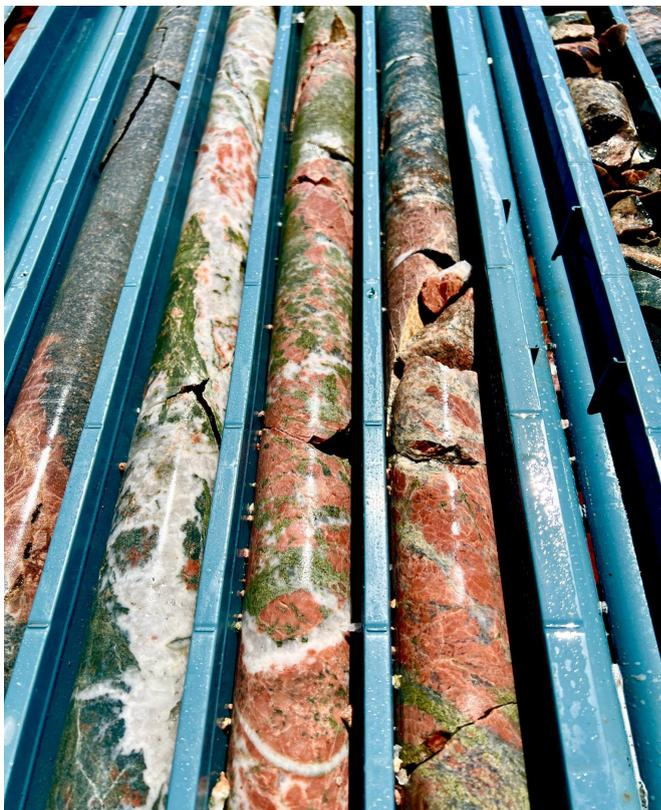
**Figure 7:** Hole WARDH073 intense Potassic alteration associated with late calcite infill (from 980m)
