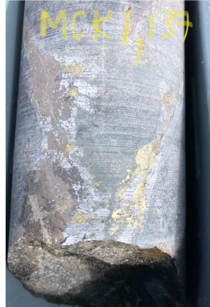
Core from the Lachlan Copper's first drill hole ("MCK1"), at Malachite Creek prospect on EL8758. The pictured core shows chalcopyrite (copper) mineralisation with pyrrhotite.
