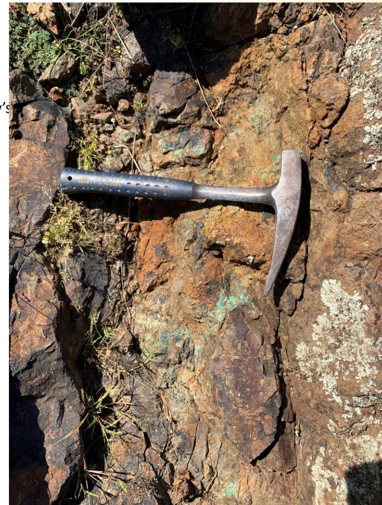
Malachite (copper mineralisation) on surface at outcrop on EL8758. This occurrence was a factor in locating MCK 1 DD hole
