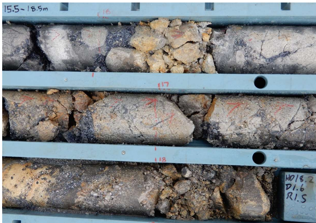
Fig 8 HQ Core photo hole 22CAEDD0010, 15.5m-18.2m Chalcocite-pyrite argillized infill breccia , dominated by argillised diorite clasts. Supergene zone 15.5m-18.5m assays 3m @ 2.45% Cu,0.22 g/t Au, 9.45 g/t Ag, 6.92 % S.
