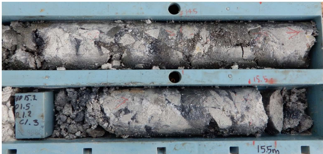
Fig 7 HQ Core photo hole 22CAEDD0010, 14m-15.5m Chalcocite-pyrite argillized infill breccia , dominated by argillised diorite clasts. Supergene zone 13m-15.5m assays 1.5m @ 1.29% Cu,0.56 g/t Au, 24.6 g/t Ag, 7.57 % S.
