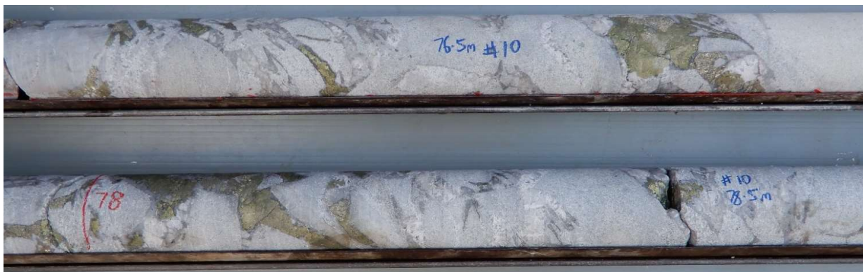
Fig 10 HQ Core photo hole 22CAEDD010, Two sections 76.5m (upper split), 78m (lower split), Chalcopyrite -pyrite, calcite-quartz infill in diorite-hornfels breccia. Primary zone 76m-79m assays 3m @ 1.79% Cu, 0.50 g/t Au, 24.9 g/t Ag, 3.66 % S.
