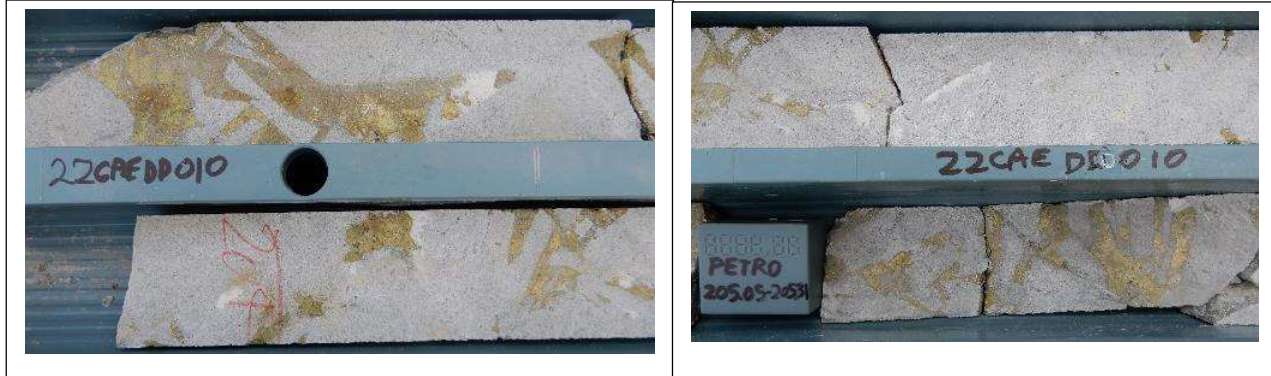
Fig 12 HQ Core photo hole 22CAEDD010, 203m-205m (LHS) ; 205m-206m (RHS) Chalcopyrite -pyrite quartz calcite infill in diorite dominated breccia. Primary zone 203m-206m assays 3m @ 2.31% Cu, 0.43 g/t Au, 40.6 g/t Ag, 5.5 % S.
