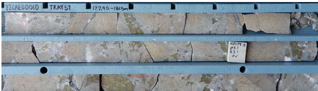
Fig 11 HQ Core photo hole 22CAEDD010, 177.0m-180m Chalcopyrite -pyrite infill in diorite dominated breccia. Primary zone 177m-180m assays 3m @ 1.53% Cu, 0.49 g/t Au, 23.2 g/t Ag, 6.06 % S.
