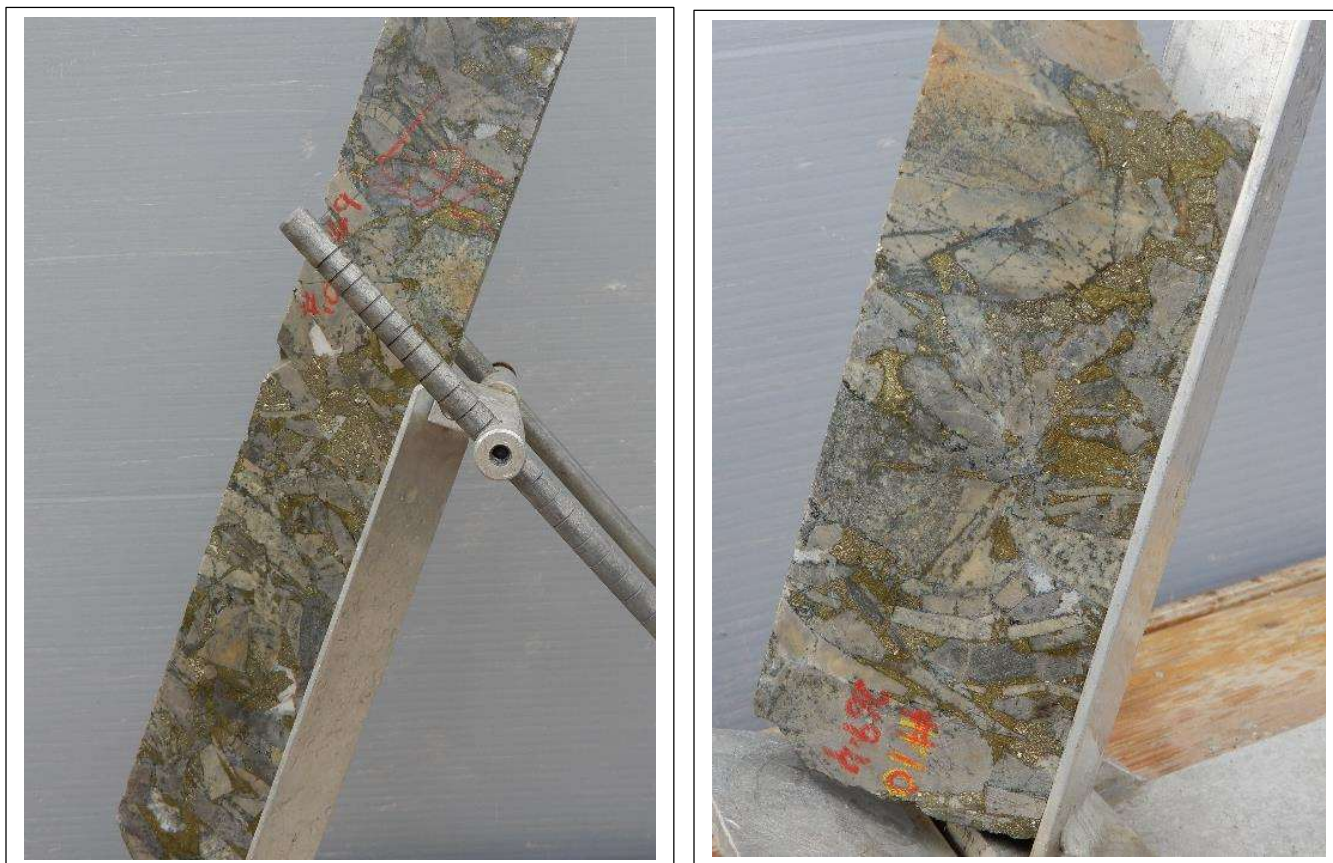
Fig 14 HQ Core Photo in core frame oriented relative to actual drillhole surveyed position, CAE hole # 10, 268.9-269.3m (LHS) ; 269.3m-269.4m (RHS). View looking to north east, hole drilling inclined 69 degrees to a magnetic bearing (azimuth) of 315 degrees ie north west. Hole # 10 drilling down the long axis of the breccia body, with drillhole cutting slabby clasts of hornfels, diorite and porphyry at high angle. Prominent chalcopyrite pyrite calcite quartz as infill between clasts. Primary zone 269m-270m assays 1m @ 3.03% Cu, 0.64 g/t Au, 40.6 g/t Ag, 9.4 % S
