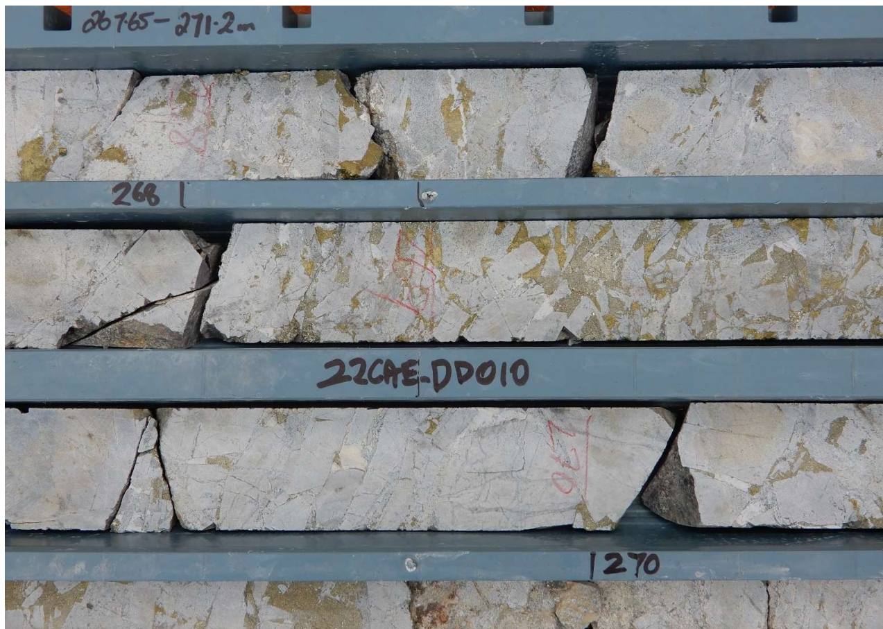
Fig 13 HQ Core photo hole 22CAEDD010, 267m-271m Chalcopyrite -pyrite quartz calcite infill in hornfels dominated breccia. Primary zone 267m-271m assays 4m @ 1.95% Cu, 0.34 g/t Au, 30.3 g/t Ag, 7.3 % S.
