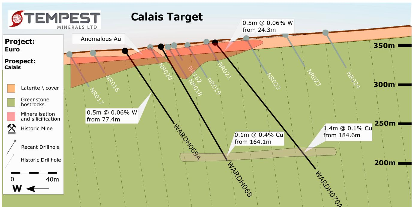
Figure 04: Cross-section through WARDH68-WARDH70A highlighting polymetallic mineralisation
