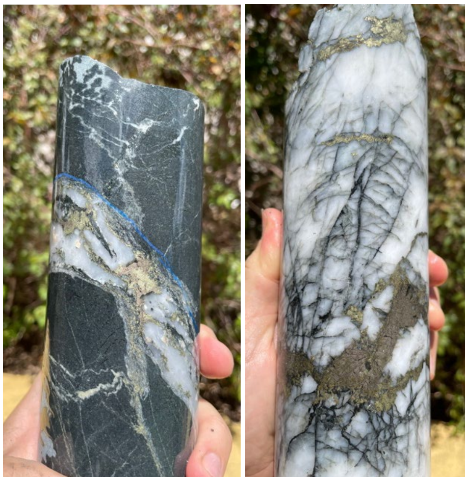
Figure 9. BTDD004 (364.9m, left). Quartz-pyrite-chalcopyrite vein. BTDD004 (376.8m, right). Buck quartz-chalcopyrite-pyrite-pyrrhotite fracture infill vein.
