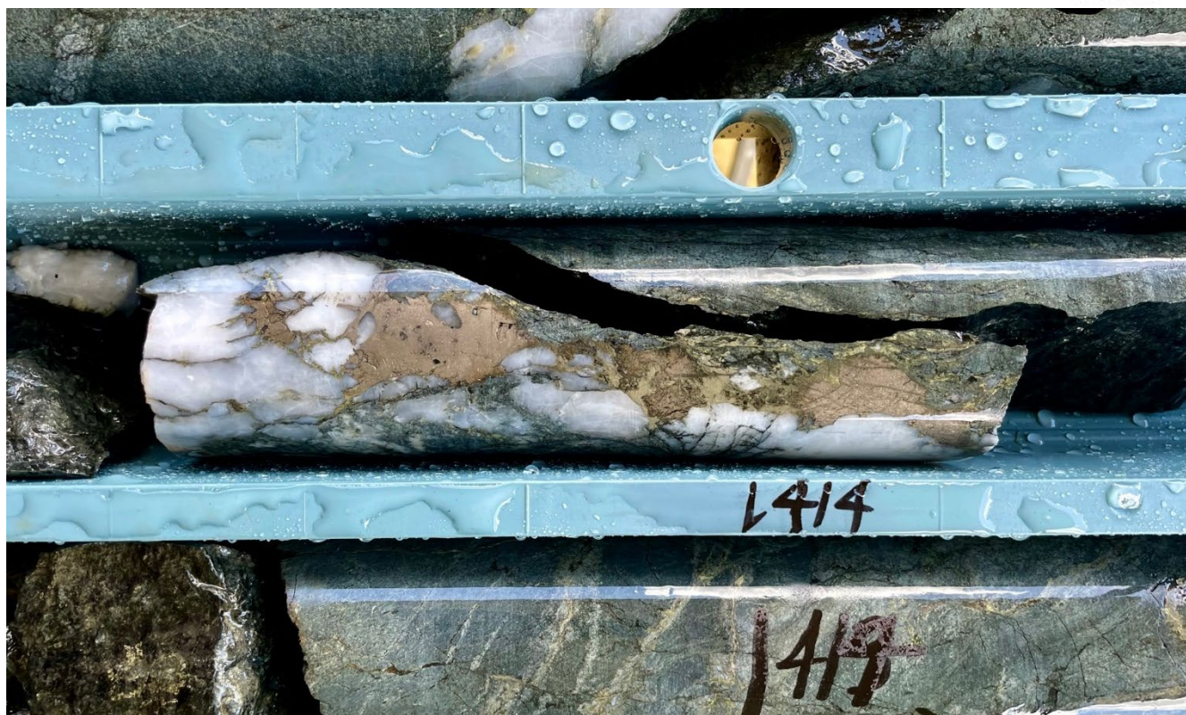
Figure 8. BTDD004 (412.9m). Buck quartz vein with massive pyrrhotite-pyrite-chalcopyrite infill.
