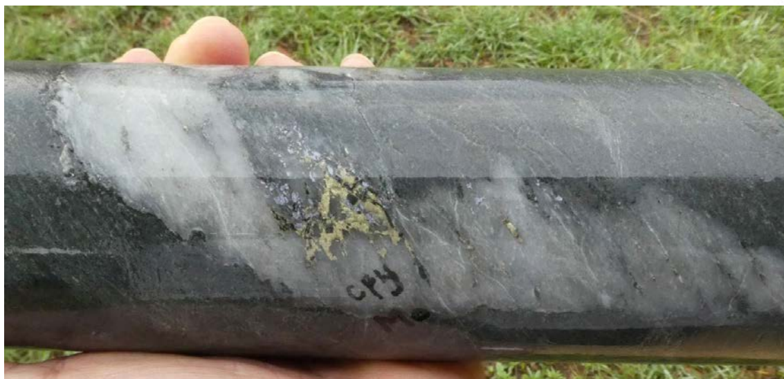
Figure 10. Deformed granular quartz vein with molybdenite along walls and internal chalcopyrite (BTDD004, 120.3m). Several such veins intersected in BTDD004 are interpreted as possible A or B Type veins within a porphyry system.
