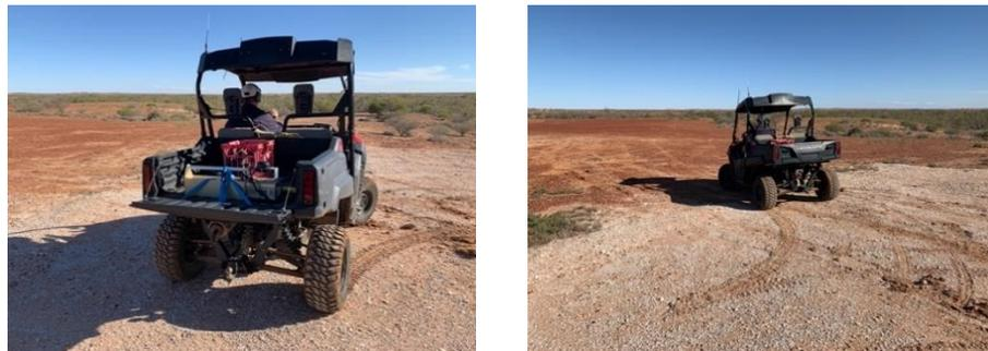
Figure 2: Buggy loaded with radiometric survey equipment
