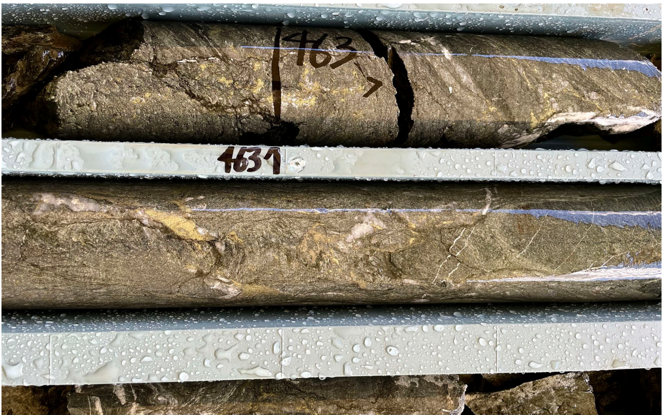
Figure 7. BTDD004 (463m). Deformed and brecciated metavolcanics with strong quartz-carbonate-pyrite-chalcopyrite veining and fracture infill.
