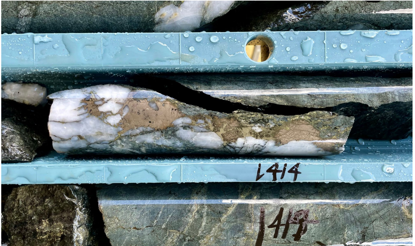
Figure 6. BTDD004 (412.9m). Buck quartz vein with massive pyrrhotite-pyrite-chalcopyrite infill.
