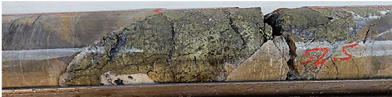
Fig 7 HQ Core photo hole 21CAEDD004, 52.5m. chalcopyrite rich infill in clast supported hornfels breccia. Primary zone 52m-53m assays 1m @ 2.7% Cu, 7.9 g/t Au, 50 g/t Ag . (approx. 1.5 oz/t Ag)..
