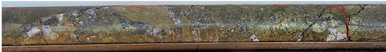
Fig 8 HQ Core photo hole 21CAEDD004, 53 to 53.5m-. infill of chalcopyrite (golden) ,pyrite (brassy), carbonate (white) quartz (glassy) in clast supported hornfels breccia. Primary zone 53m-54m assays 1m @ 5.35% Cu, 5.71g/t Au, 88 g/t Ag. (approx. 3 oz/t Ag).
