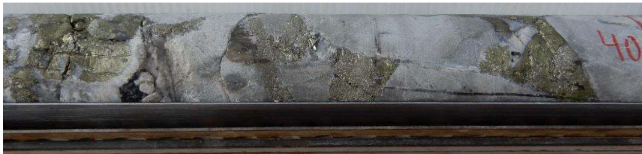
Fig 6 HQ Core photo hole 21CAEDD004, interval 40m to 40.2m. Pyrite and chalcopyrite + quartz-carbonate infill in clast supported hornfels breccia. Primary zone 40m-41m assays 1m @ 2.62% Cu, 1.36 g/t Au, 46 g/t Ag . (approx. 1.5 oz/t Ag).
