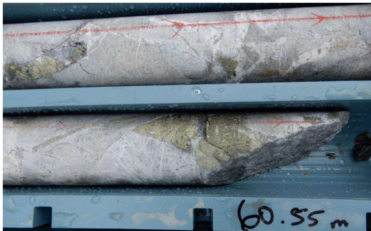
Fig 11 HQ Core photo hole 21CAEDD004, section 59m to 60.5 m, infill of chalcopyrite rich section of clast supported hornfels breccia. Primary zone 59m-61 assays 2m @ 1.32% Cu, 1.42 g/t Au, 32 g/t Ag (1 oz/t Ag) .
