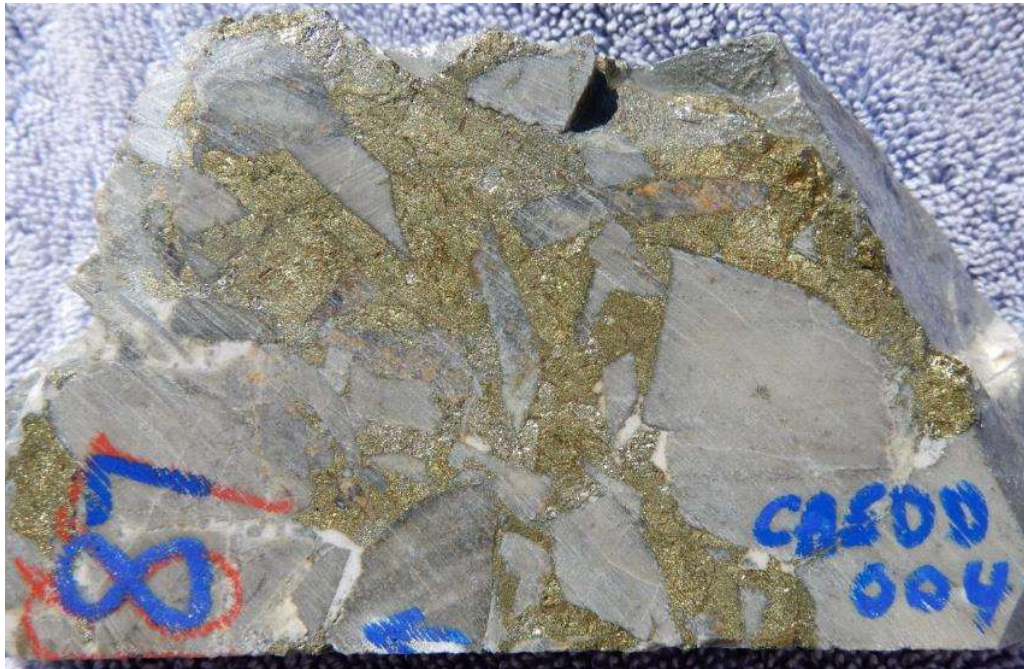
Fig 12 HQ Core photo hole 21CAEDD004, at 87m, infill of chalcopryite, pyrite in clast supported hornfels breccia. 87m-88 assays, 1m @ 1.99% Cu, 0.14 g/t Au, 39 g/t Ag (1oz/t Ag).
