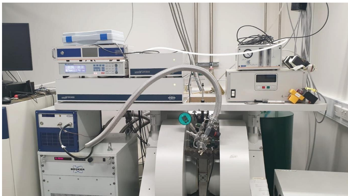
Image 2. Electron spin resonance setup to validate qubit robustness.
