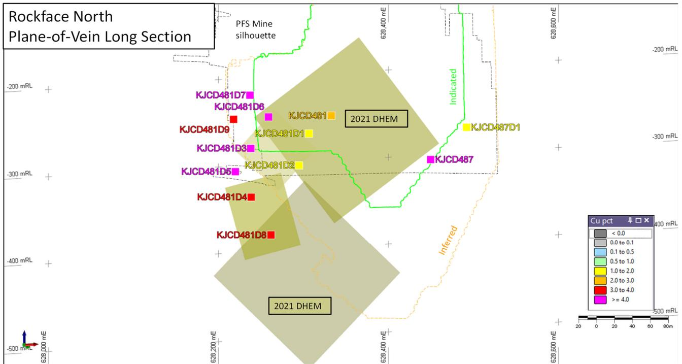
Figure 1: Long Section of Rockface North showing the position of the 2021 drill intersections in relation to the 2020 resource model and PFS mine plan silhouettes. Also shown are the DHEM conductor models interpreted from the DHEM surveys of KJCD481D3 and KJC481D4.
