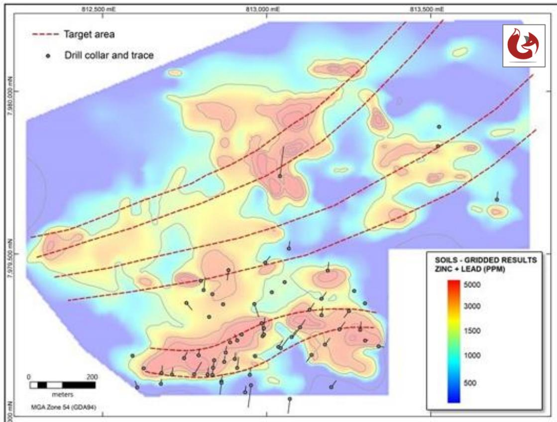
Figure 4: Soil sampling (by Minad, 1960s) at Eveleigh showing location of historical drilling
