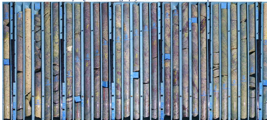
Photo 1. Drill hole WCS007 NQ core showing 24.15 metre mineralised intercept
