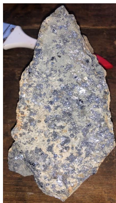
Photo 2: Webbs Consol Main Shaft Specimen showing coarse galena mineralisation
