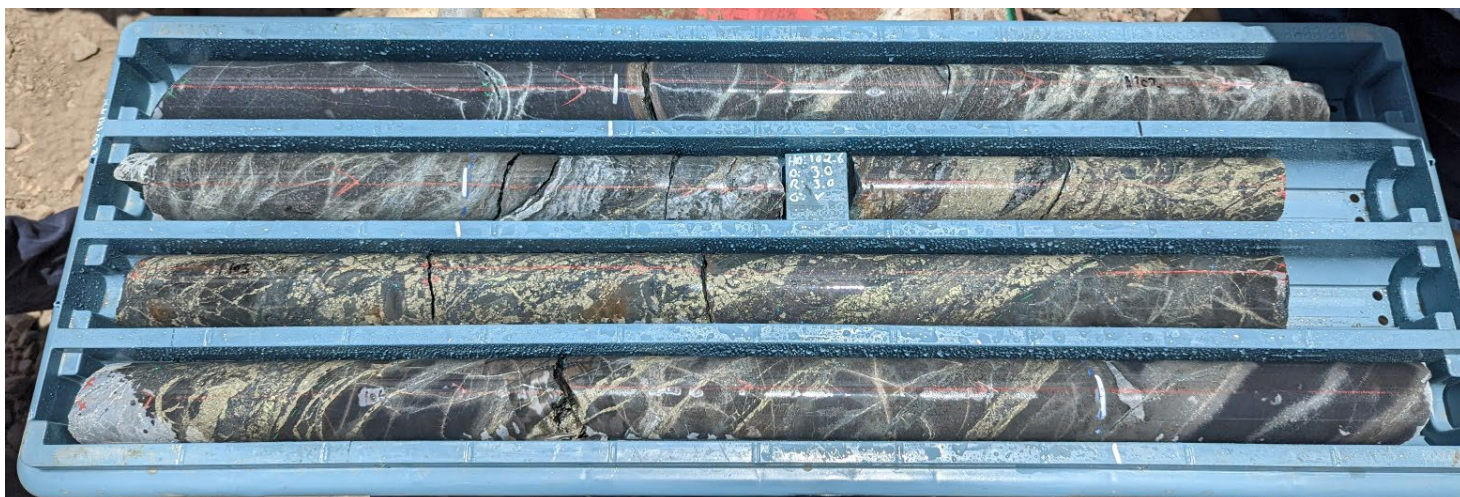
Figure 3. Two metre chalcopyrite – pyrite – magnetite zone intersected at 102m depth in BNDD003.
