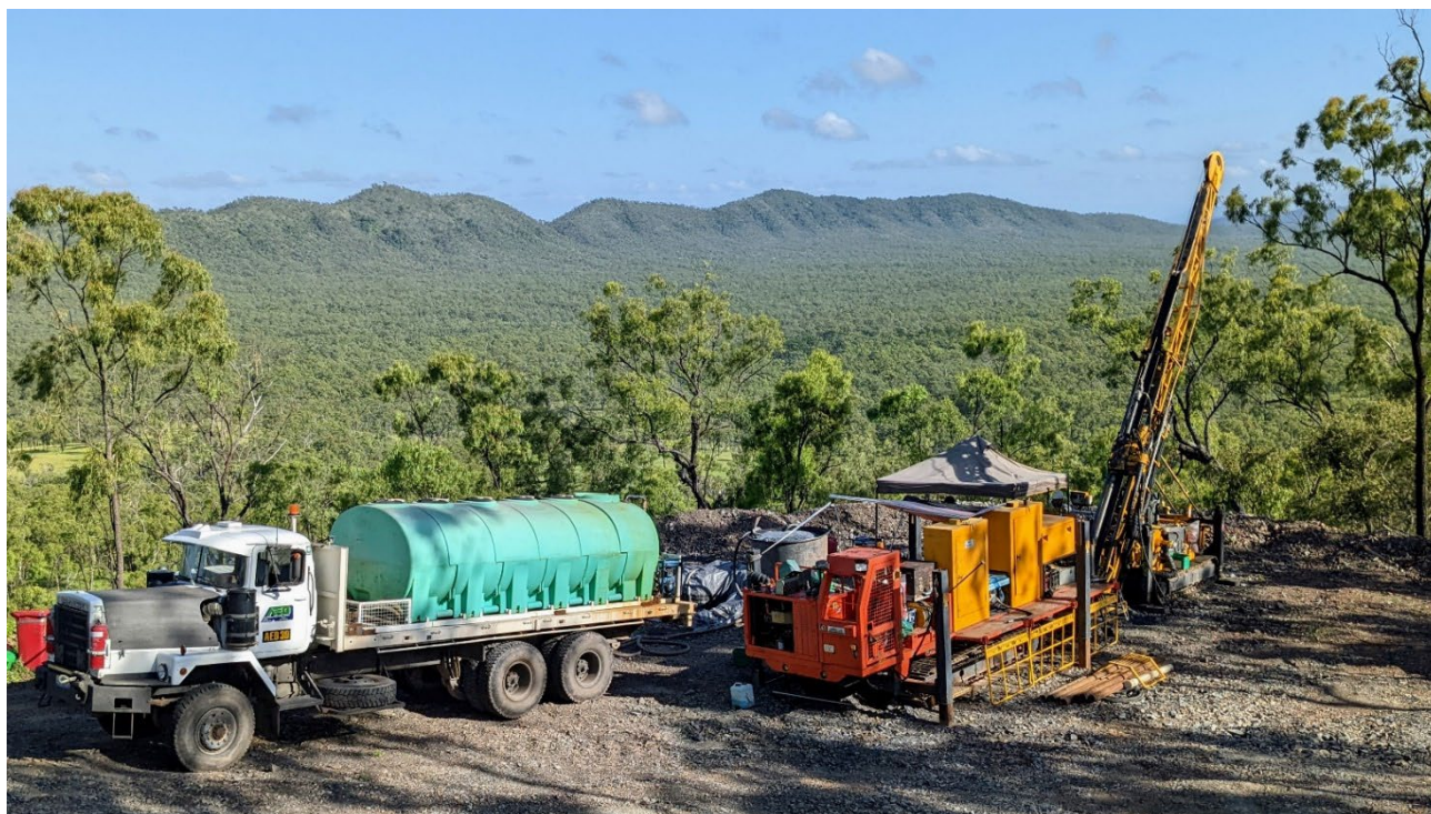
Figure 2. Diamond rig drilling BNDD003 at Rogers testing a coincidental geophysical and soil anomaly.
