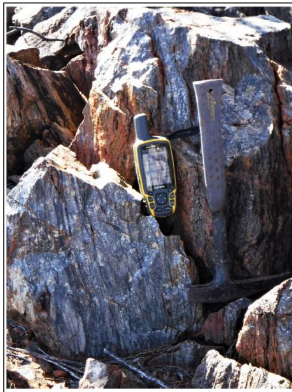
Figure 4: Quartz mylonite in sheared ultramafic host (rock-chip sample GNR002). The dark septa consist of a fine-grained mixture of iron oxides and phyllosilicates with fine box-work textures after oxidised pyrite.
