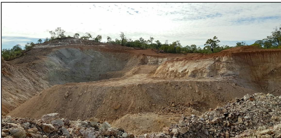
The below image shows the northern extension of the existing open cut post blasting prior to the start of waste material being mined off to allow for the RC drill program. Two of the drill pads outside the blast area can be seen highlighted in green & CCGC235 for reference to next image.
