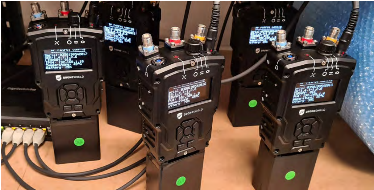
Image: RfPatrol MKII™ units undergoing final QA testing prior to shipment
