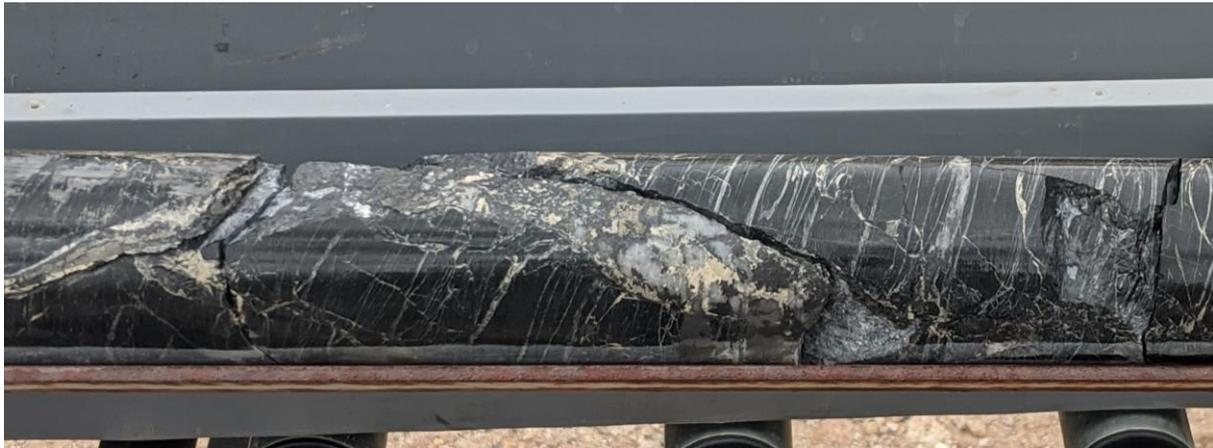
Figure 5. Semi massive sphalerite-pyrite veins and stringers overprinting quartz within silicified shale (~640m).
