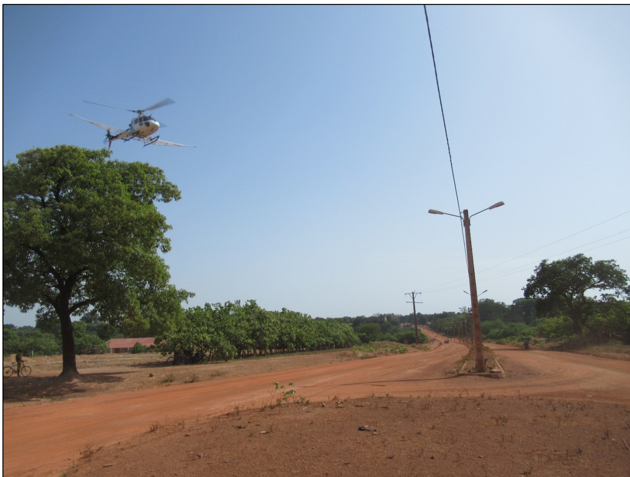
Figure 2: Helicopter flying at low altitude collecting aeromagnetic/ radiometric data
