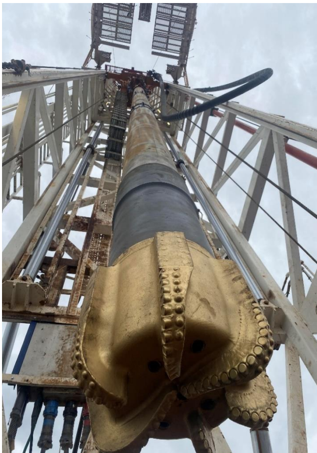
Carpentaria-1 drilling with casing
