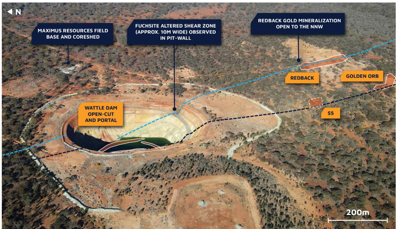
Figure 1. View looking East: Wattle Dam Gold Mine and Maximus prospects to the SSW. Dashed lines represent interpreted shear zones. Note that the actual geometry of the S5 prospect is not well defined and is the focus of the upcoming RC drilling programme. The representation of mineralisation in the Wattle Dam open-cut is now mined-out.
