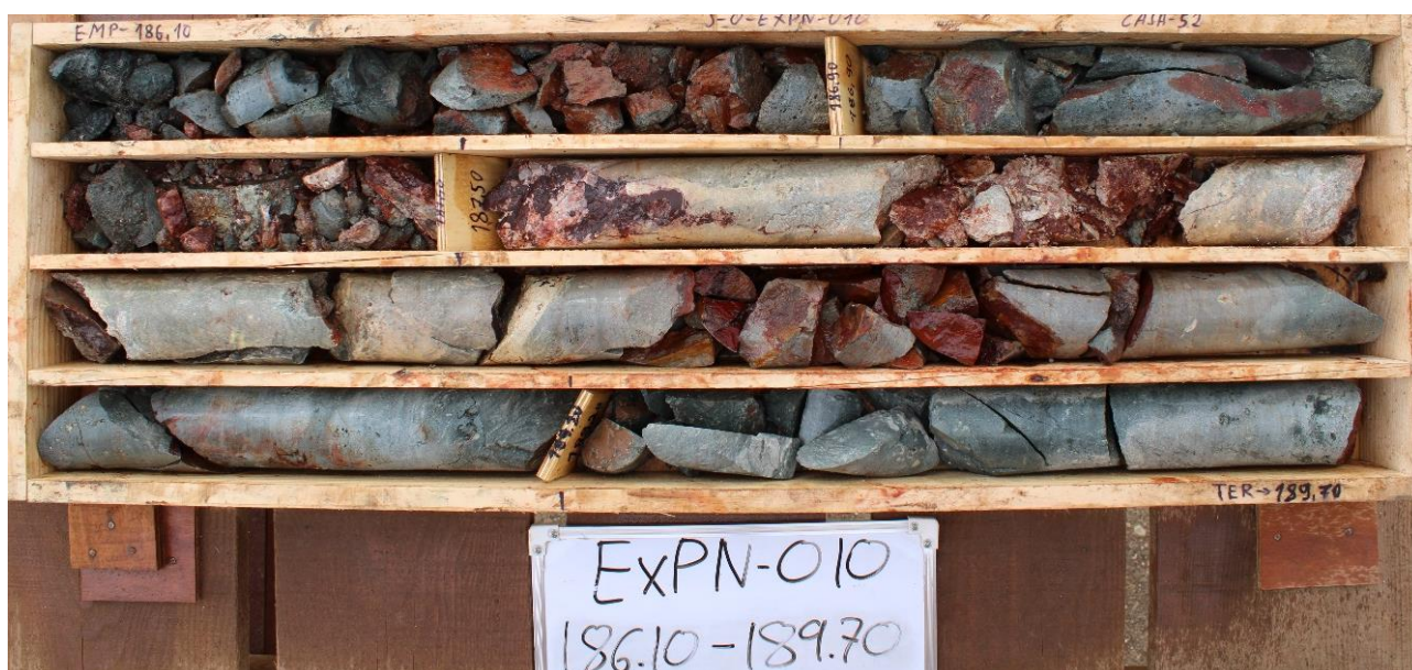
Figure 2. Expn_010:- Fresh to transitional HQ diamond drill core from 186.1 – 189.7m.
