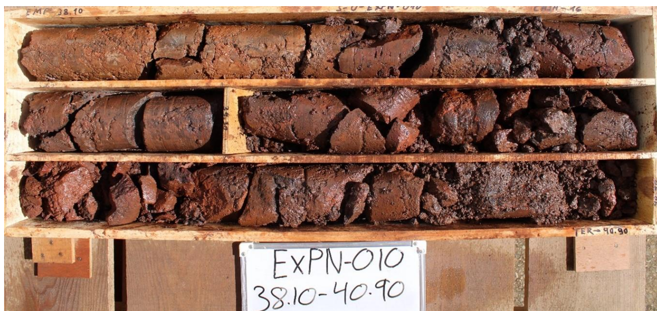
Figure 1. Expn_010:- Heavily oxidised PQ diamond drill core from 38.1 – 40.9m.
