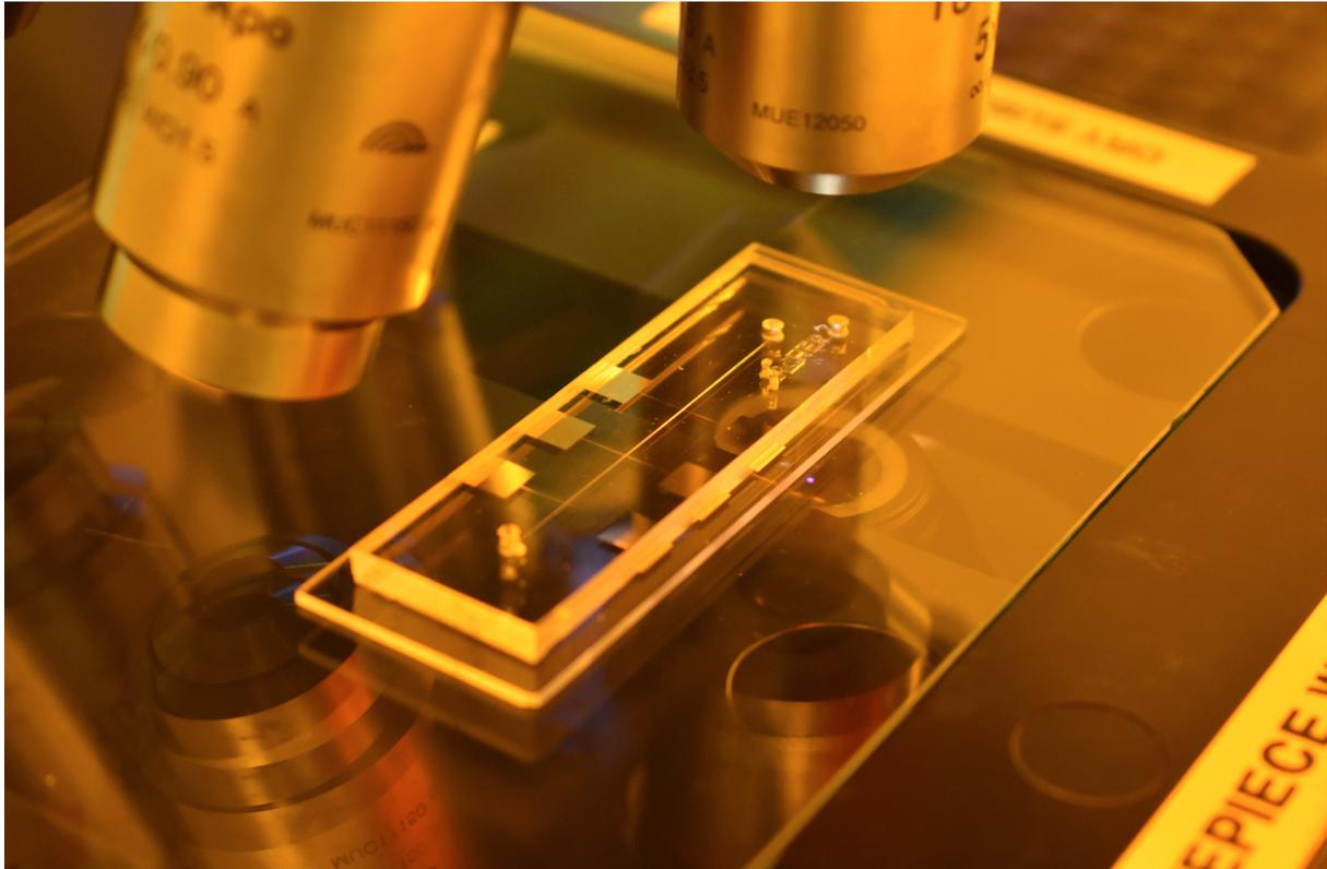
**Image 1. Building Archer's A1 Biochip™.** Archer's biochip development involves miniaturising medical lab tests onto an integrated circuit, a single chip, that is only a few millimetres in size. The chip includes a number of functional areas and componentry, including microfluidic channels and active biosensing areas – all smaller than the thickness of a human hair.
