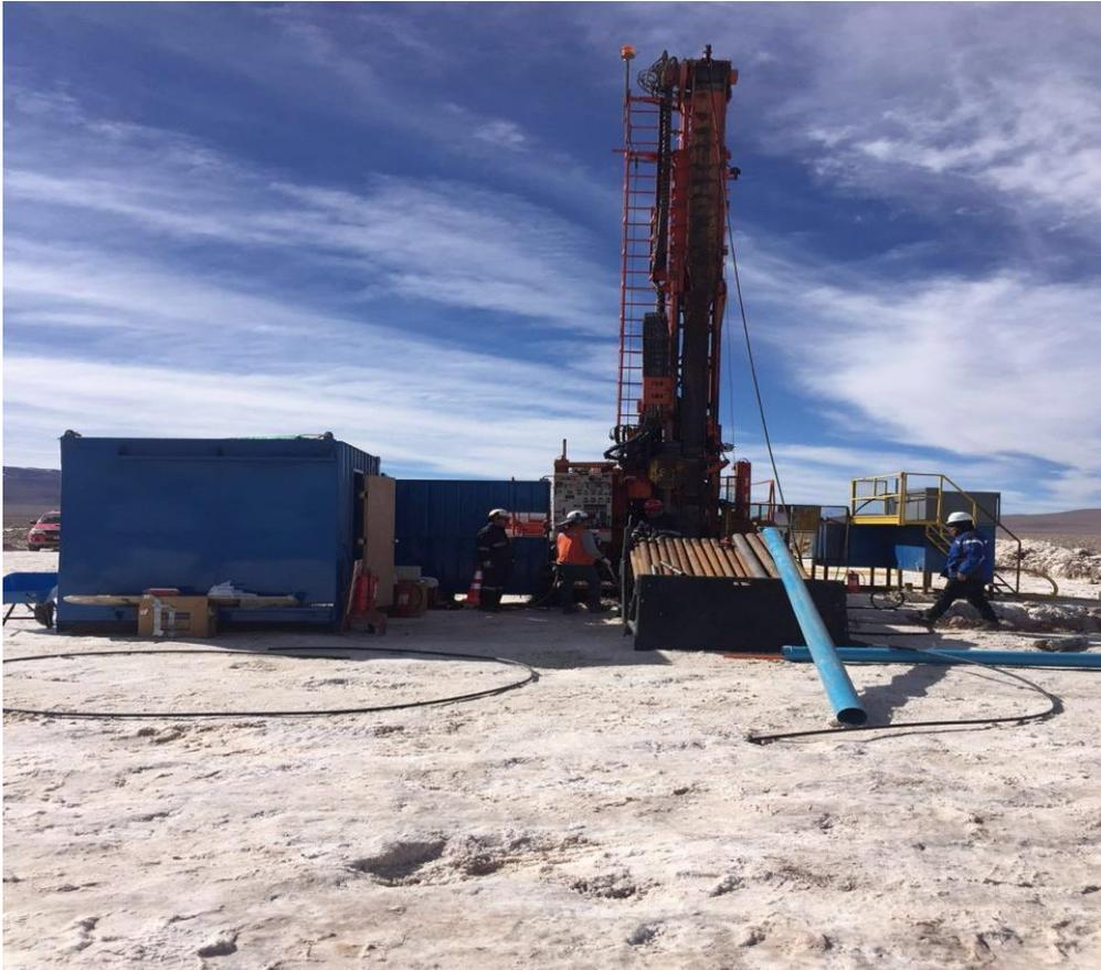
**Figure 3 - Drilling of the S19 borehole to 362 m in the 2018-19 drilling program**
