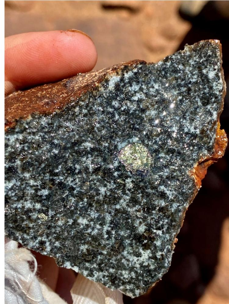
*Coarse grained mafic intrusion showing high tenor three phase disseminated and blebby sulphides comprised of chalcopyrite, pentlandite and pyrrhotite*
