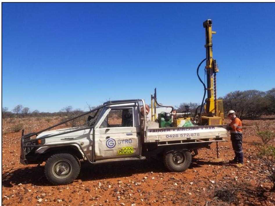
**Figure 3 – Auger drilling at Westar’s Winjangoo Project**
