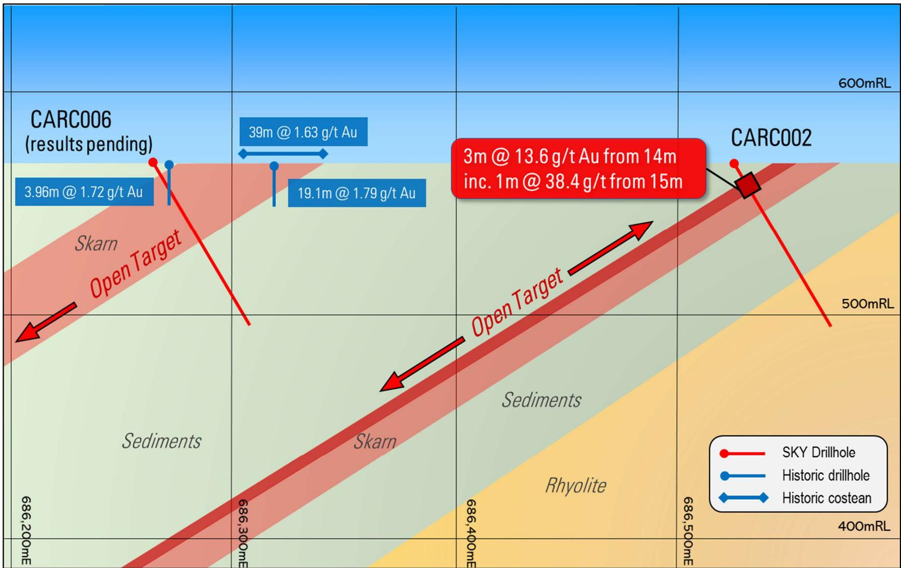
Figure 2 - Caledonian Target - Schematic cross section - 6,130,000mN
