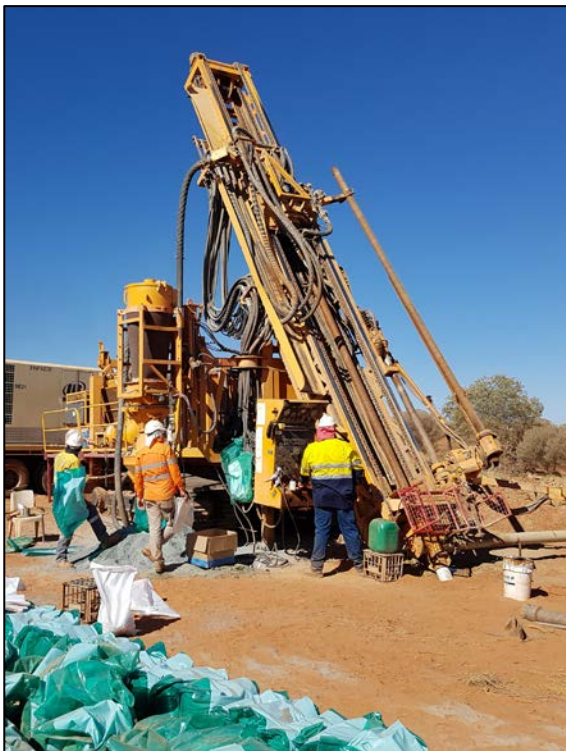
Images 1 & 2: RC rig drilling VHBR00010 & Diamond rig drilling VHBRCD0006 at PHB-1, Marymia Gold Project
