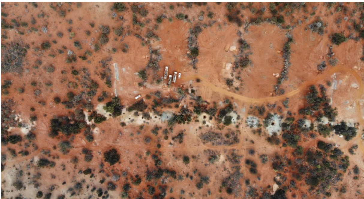
Figure 7: Drone image (north to the right) showing historical workings at Metzke's Find including additional workings to the south (left side of the image). The rig is on drill hole MZRC013 in this photo.
