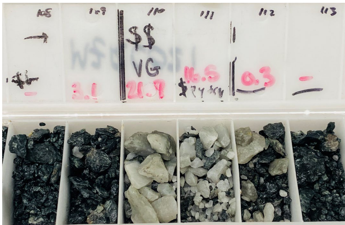
Figure 3: RC chips from MZRC021 (107-113m) showing an intercept of the lode consisting of a sugary quartz-sulphide vein with within a biotite altered structure from 108-111m grading 13.8g/t Au.
