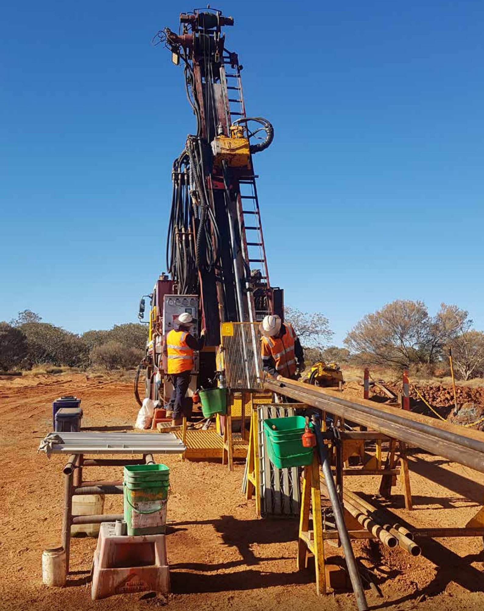
Diamond drilling at PHB-1
