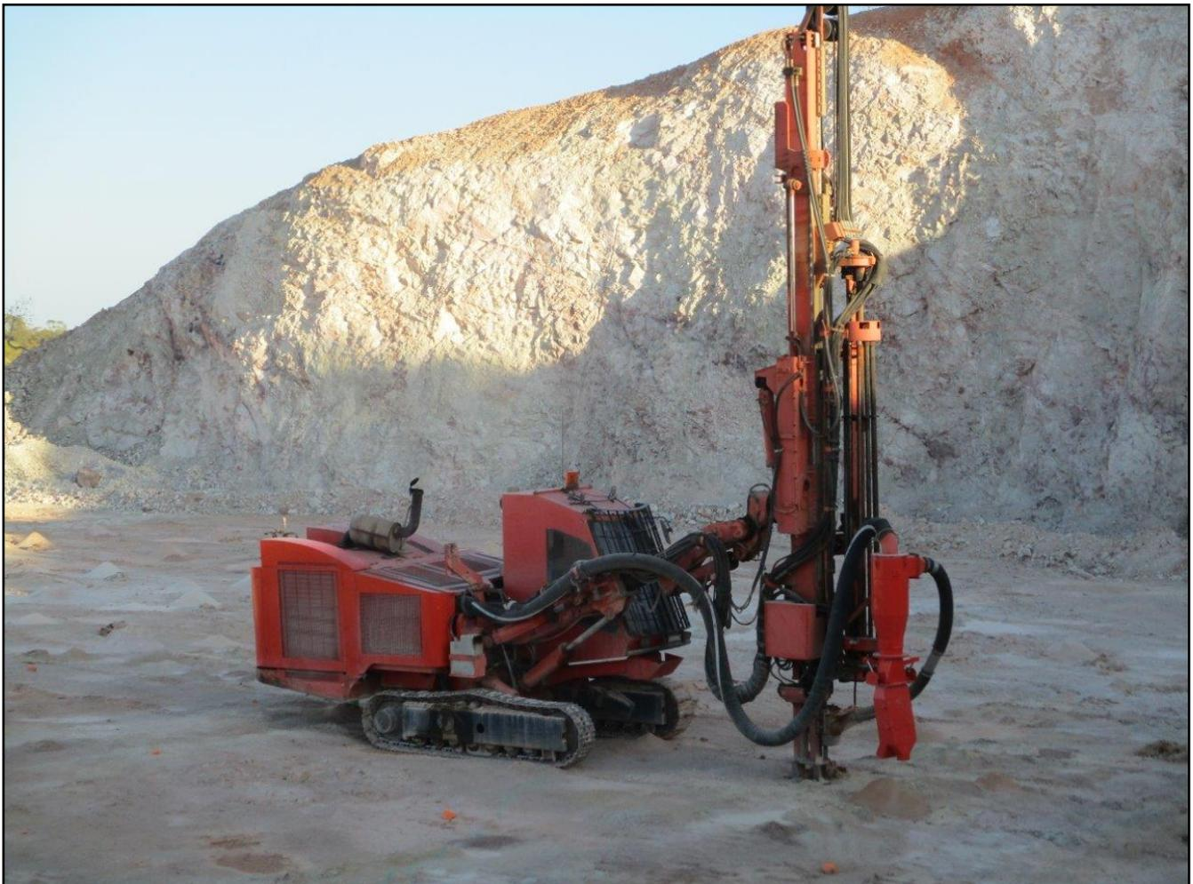
Blast hole drilling in preparation for initial blast – 16/10/2020
