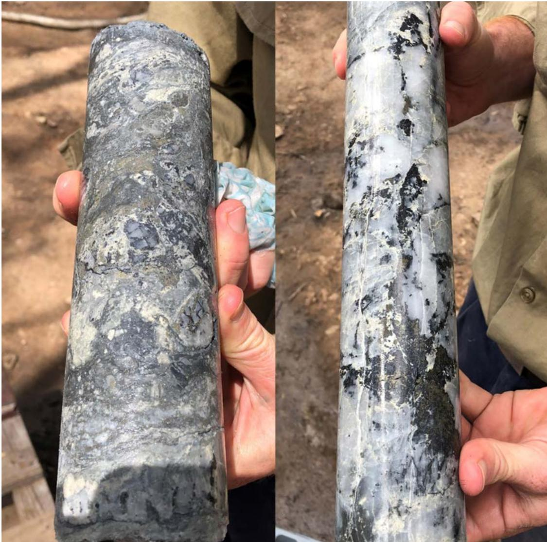
*Figure 5. Left Image - sphalerite, galena and pyrite in matrix of breccia (~695m). Right image - black sphalerite in quartz vein (~699m depth)*
