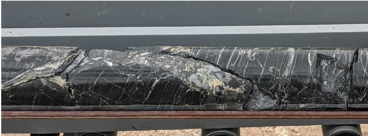
Figure 3. Semi massive sphalerite-pyrite veins and stringers overprinting quartz within silicified shale (~640m).
