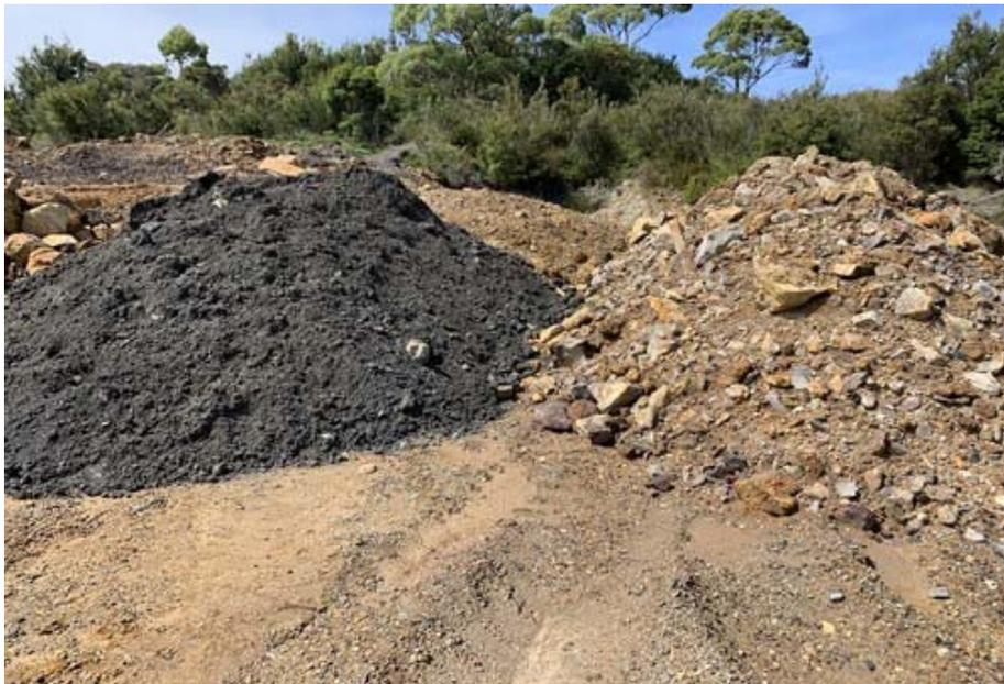
Figure 1 – Truck-load from first mining block - hanging wall shale (left) and skarn (right)
