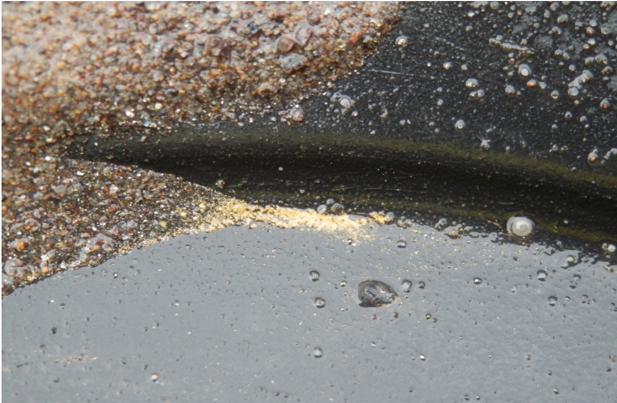
Figure 7: Visible Au tail in panned concentrate from crushed Piccadilly lode.
