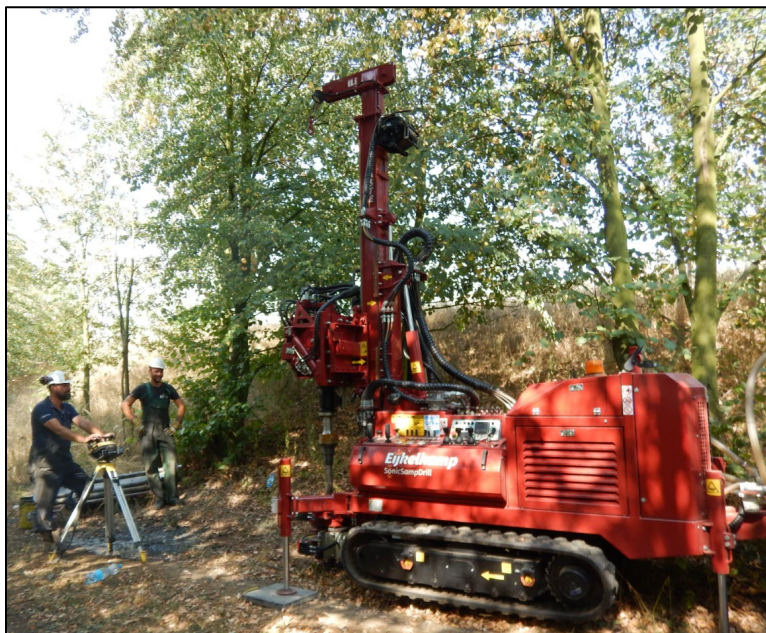
Photo 10-2: Eijkamp SonicSampDrill SRS Used for 2018 Sonic Drilling Investigation
