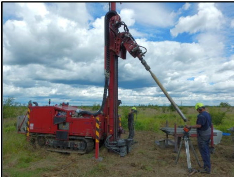
Photo 10-1: Showing Eijkelpamp SonicSampDrill B.V. and Drill Crew
